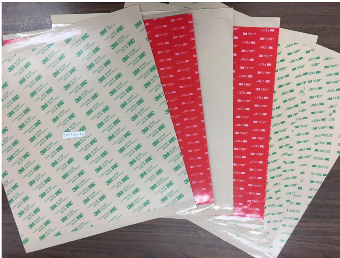
Figure 4.3.1: (Seven different types of acrylic polymer double-sided tapes from 3M were ordered. Four of these tapes were used to investigate their optical coupling performance.
