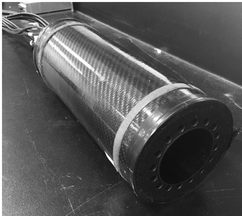
Figure 2.6.3: The first-generation PET insert, consisting of a ring of 16 detector modules mounted in a light-tight enclosure.
