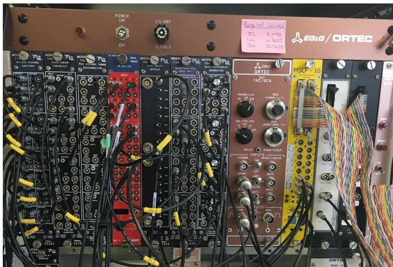
Figure 3.2.1: NIM chassis containing several NIM modules for data acquisition.
