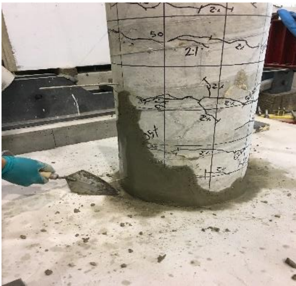
(c) Patching with mortar
