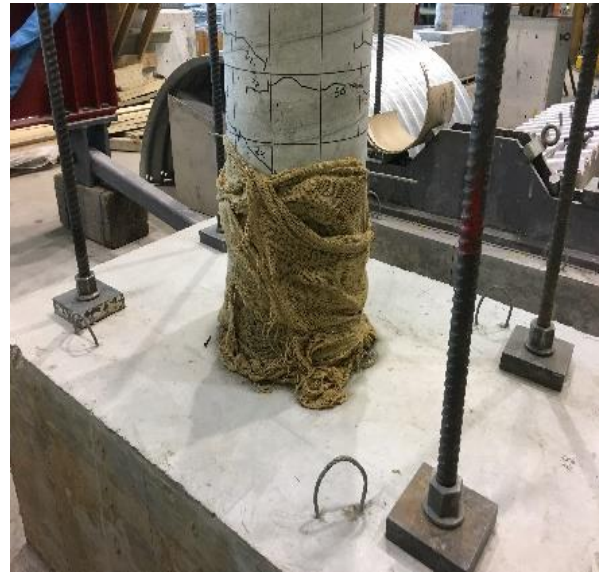
(d) Curing with wet burlap
