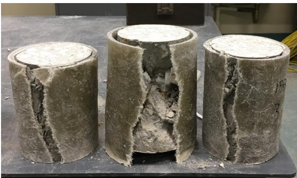
(b) Cylinders after test
