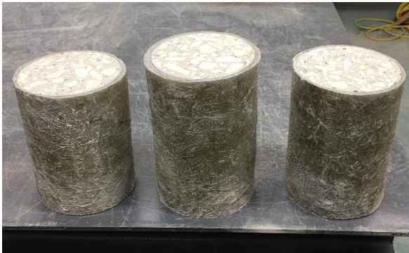
(a) Strengthened cylinders
