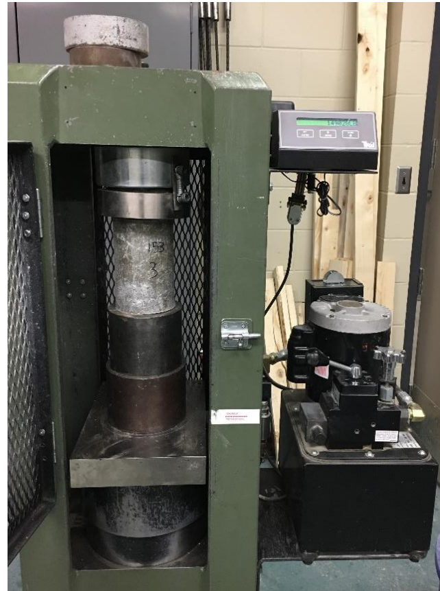
(c) Testing of strengthened cylinders
