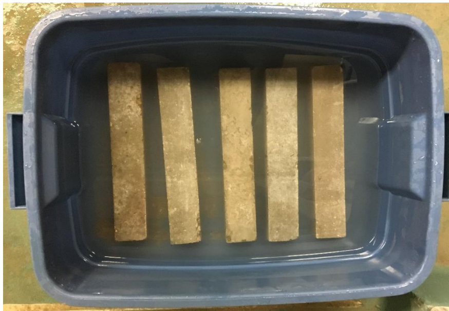
Fig. 3. 1: Incremental aggression of the sulfuric acid exposure: phase I, II and III
