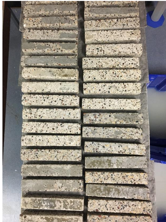
Fig. 3. 5: Drying the specimens in laboratory conditions after taking them out of the solution.
