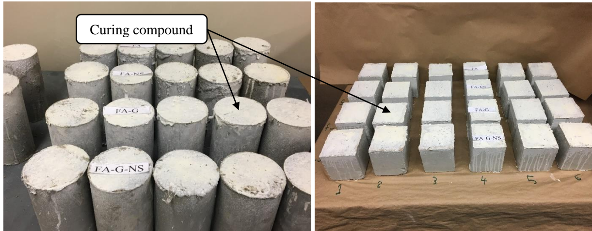
Fig. 3. 9: Spraying the top surfaces of the mixtures after casting by a curing compound.
