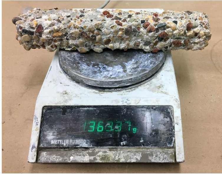
Fig. 3. 6: Weighing the specimens after drying to calculate the relative mass change.
