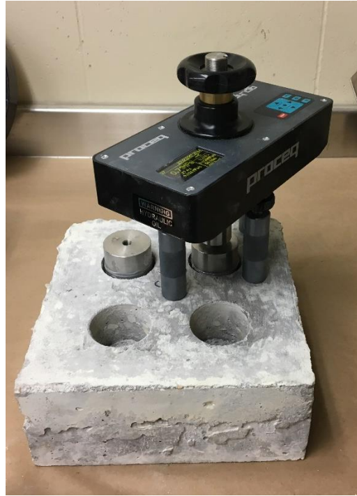
Fig. 3. 14: The pull-off test.
