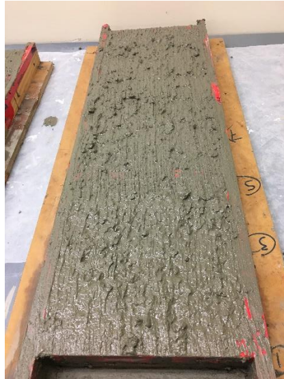
Fig. 3. 10: Wire brushing the surface of the substrate slabs after casting.
