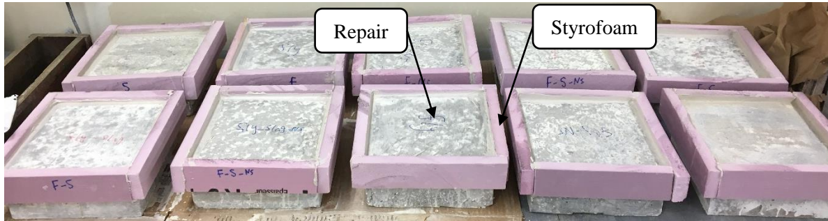
Fig. 3. 12: Test set-up for the slabs before ponding with the sulfuric acid solution.
