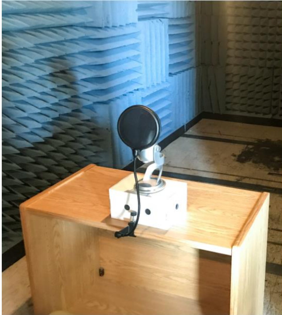
Fig. 4.11. The setup of the Blue Yeti with a pop-shield filter placed in front of it.
