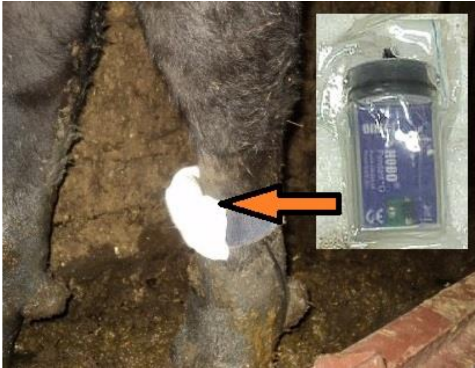
Figure 4. HOBO Pendant G accelerometer enclosed within a waterproof casing and attached to the hind leg.
