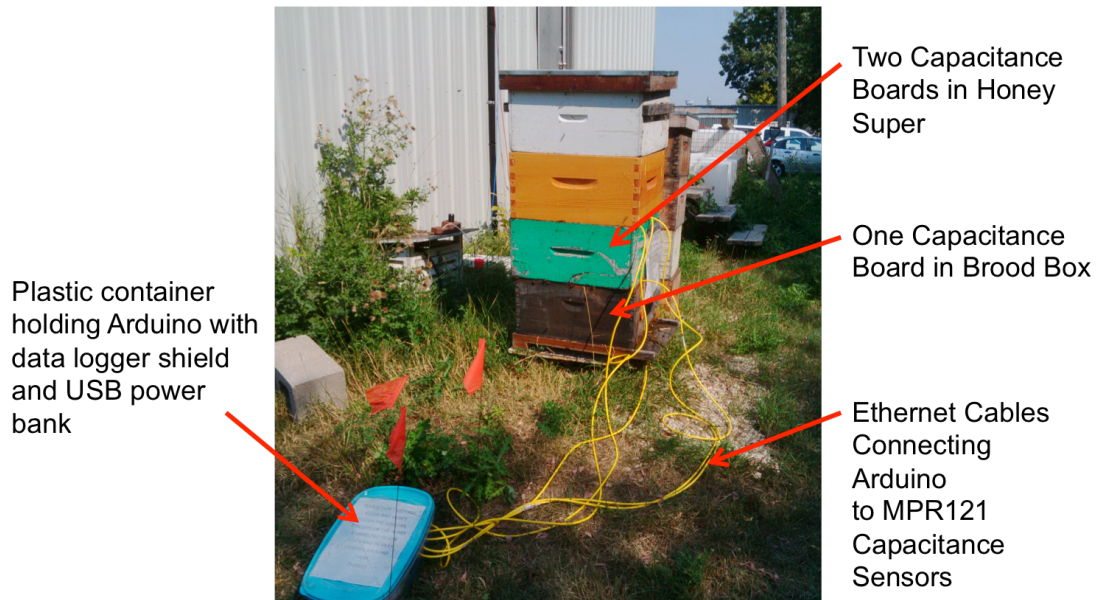
Figure 4.22 Field test set-up
