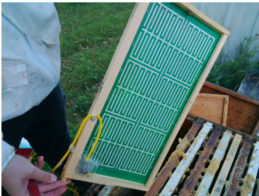
Figure 4.26 Capacitance board being removed after 29 days inside the hive
