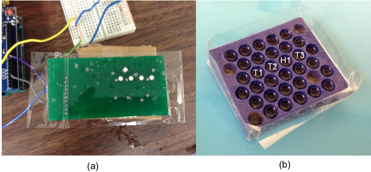
Figure 3.19 Lab heat test setup with (a) the PCB board and (b) the 3D printed comb placed such that the cells lined up as labeled with the components on the PCB
