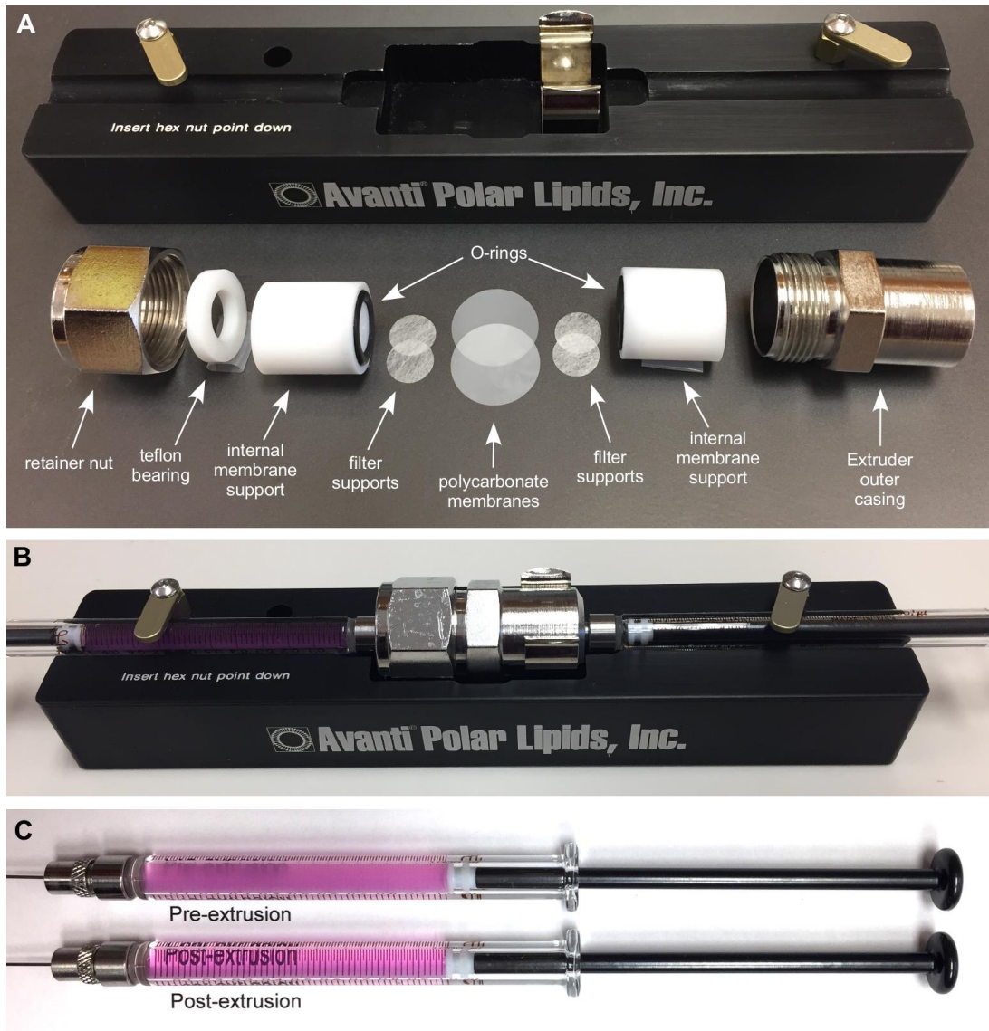
Figure 6. Overview of the Avanti Polar Lipids, Inc Mini-Extruder. A. The order of assembly of the various parts of the mini extruder. Parts are indicated by name in the image. B. The assembled extruder with a syringe full of lipid suspension on the left and an empty collection syringe on the right. C. Two syringes filled with a suspension of liposomes. The top syringe is pre-extrusion, the bottom syringe is post-extrusion. Notice the improved clarity of the suspension post extrusion (typing is legible through the glass syringe).
