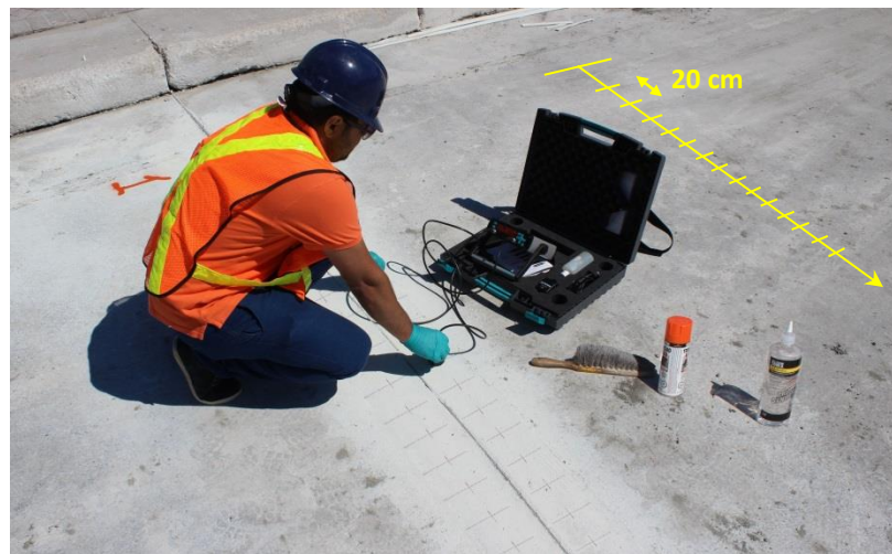
Figure 10.7: A grid was applied to the surface of a repaired joint to allow locations to be correlated with UPV measurements.
