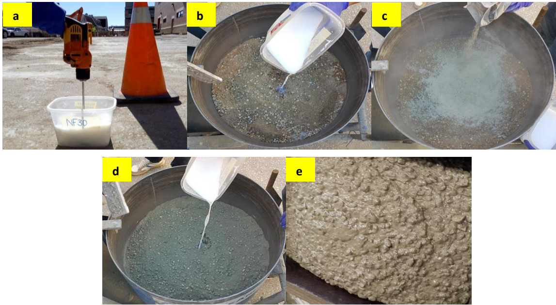
Figure 10.4: Sequence of mixing for the NMFC repairs. : (a) liquid components (water, nanosilica, and admixtures) were stirred vigorously at 1800 to 2600 rpm for 45 seconds; (b) about 15% of the liquid was added to the aggregates while mixing for 30 seconds; (c) cement and fly ash were blended with the aggregates and mixed in the mixer for 60 seconds; (d) the remaining liquid was added and mixing continued for 2 minutes; and (e) the mixture was ready for placement.
