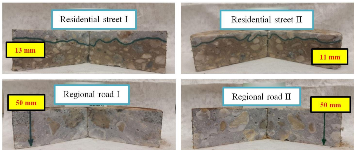
Figure 3.6: Whitish color showing the chloride penetration.
