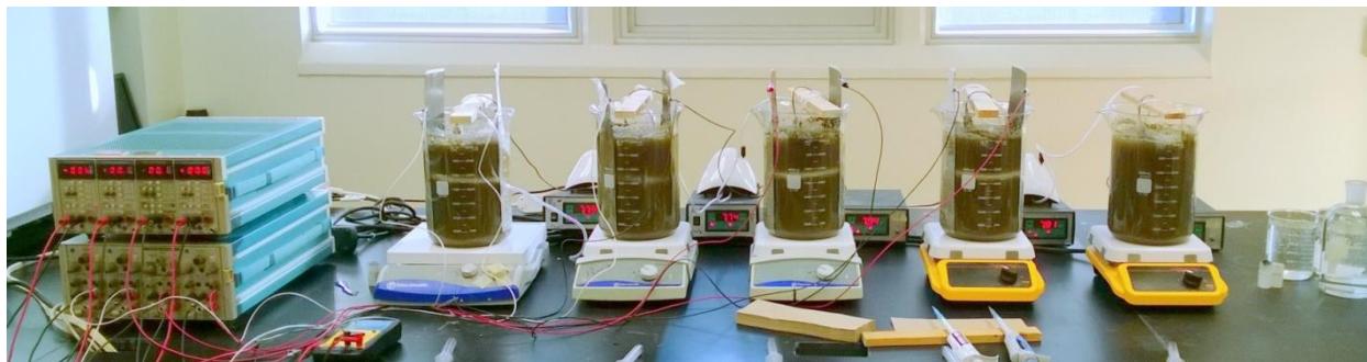
Figure 4.2: Picture of Experimental Set-Up for Short-Term Nitrifiers Exposure to Electric Current
