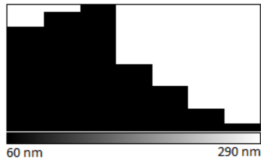
Figure 5.3. Diameter distribution of PU/CNT nanofibers obtained from analysing SEM images.
