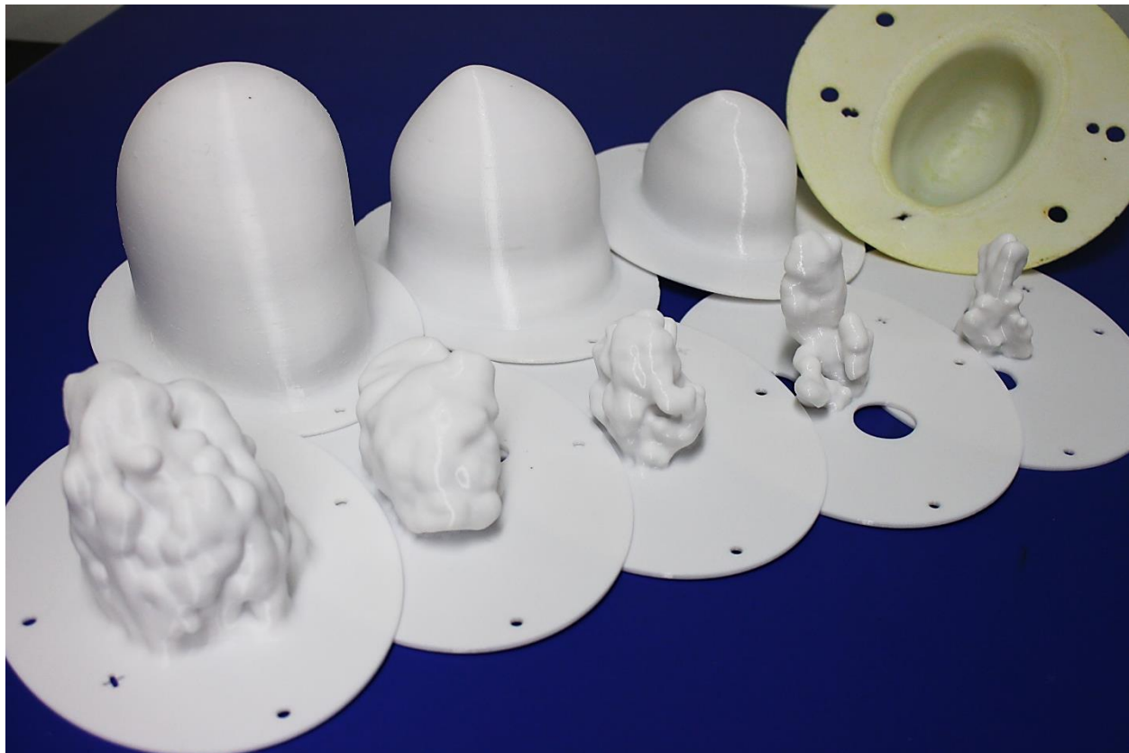
Figure 4.7-1 Array of 3D-printed phantoms. The three adipose containers (top row, white), combined with the five fibroglandular containers (bottom row) representing the diverse density and size of breasts. In the top right corner, a flipped prototype shows the inner side of an adipose container.
