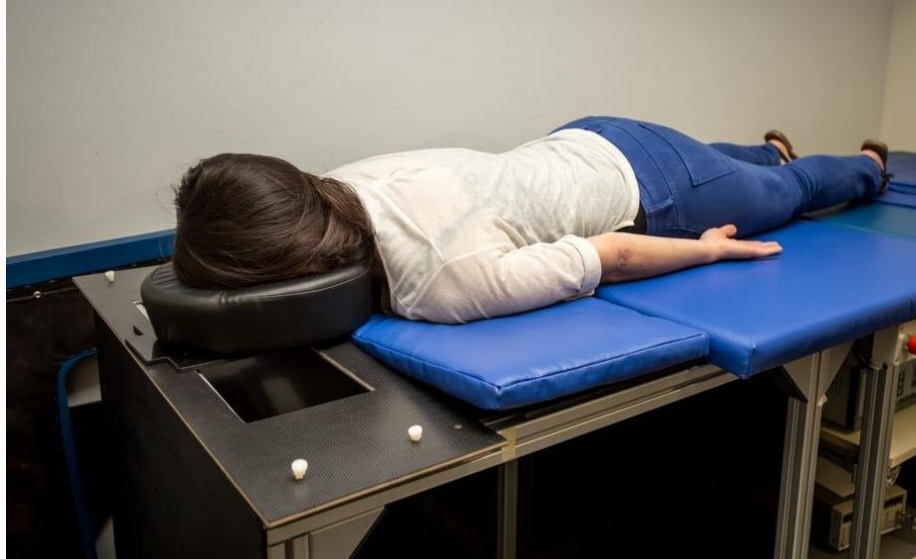
Figure 2.4-2 Volunteer above the BIRR system with the re-designed head and chest supports. A massage-like headrest supports the weight and position of the head. The headrest, in turn, lies on top of an ABS plate with a rectangular slit for air circulation. The chest area is supported by a 1-cm thick carbon-fiber support and a custom-made padded cushion, with a central aperture.
