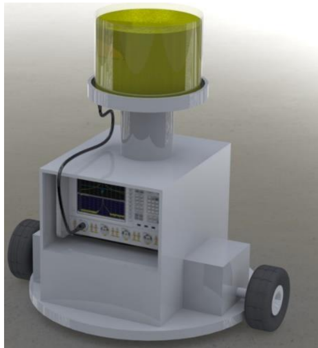
Figure 2.2-2 CAD render of discarded BMI concept #1 Microwave equipment sits below round tank for impedance matching liquids. The device rotated on its vertical axis under an inspection bed (not shown in this figure).
