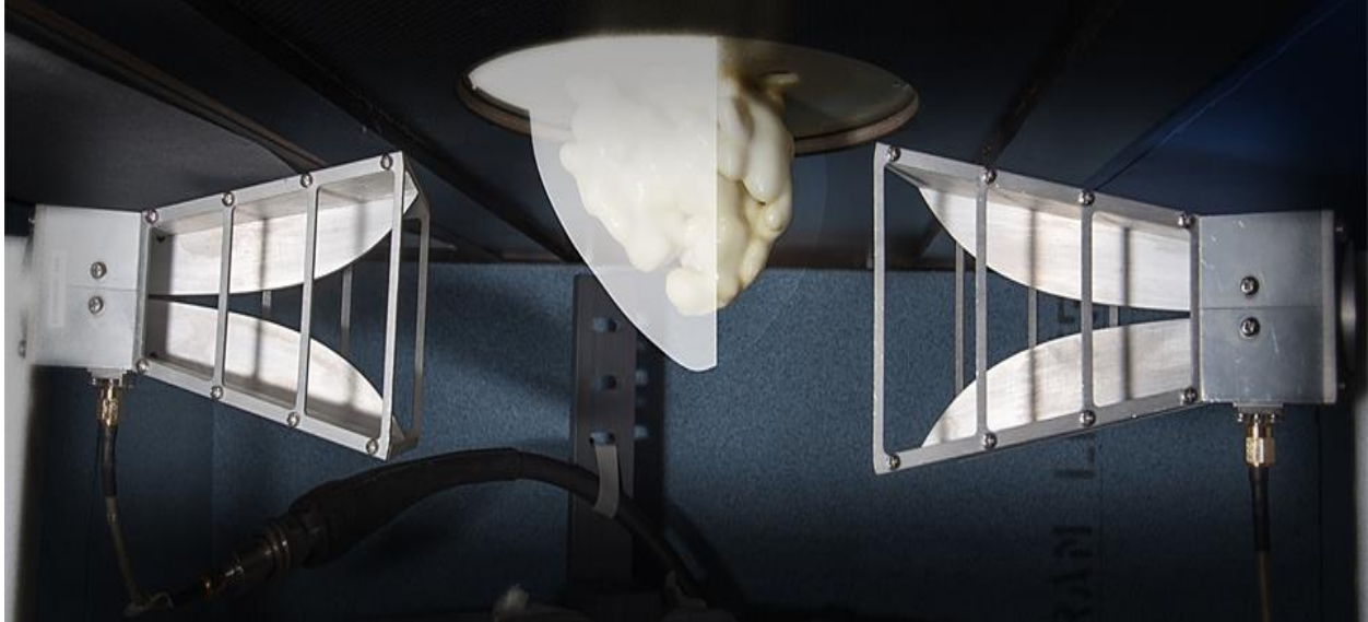
Figure 4.7-2 Class III 3D printed phantom in the BIRR imaging chamber. The photo shows half of an adipose container, with increased transparency, to show the fibroglandular insert. The opening on the base of the phantom allows for tumor inclusions to be placed close to the fibroglandular structure.
