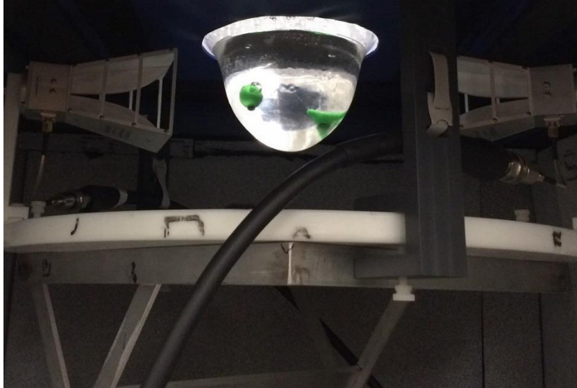
Figure 4.6-1 Photo of the CAB-D+ phantom container positioned in the imaging chamber of the BIRR. The dimensions of each container provided an approximate representation of the possible breast sizes during a clinical scan. During the BIRR pre-clinical trial (see section 2.6.3) the CAB containers served to adjust the radial position of the antennas before the patient examination. The transparency of CAB facilitates the setup of targets inside the phantom.
