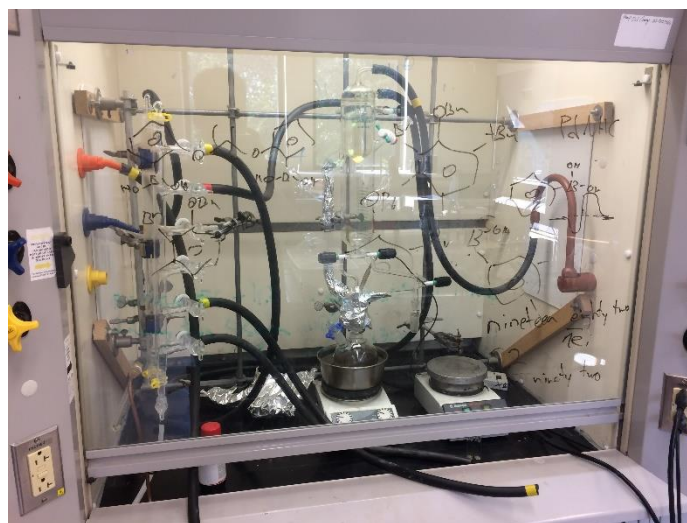
Figure 1- 7. Schlenk Technique in Budzelaar Laboratory.
