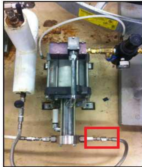
Figure 3.8 Swegelok fitting on high pressure side of booster pump
