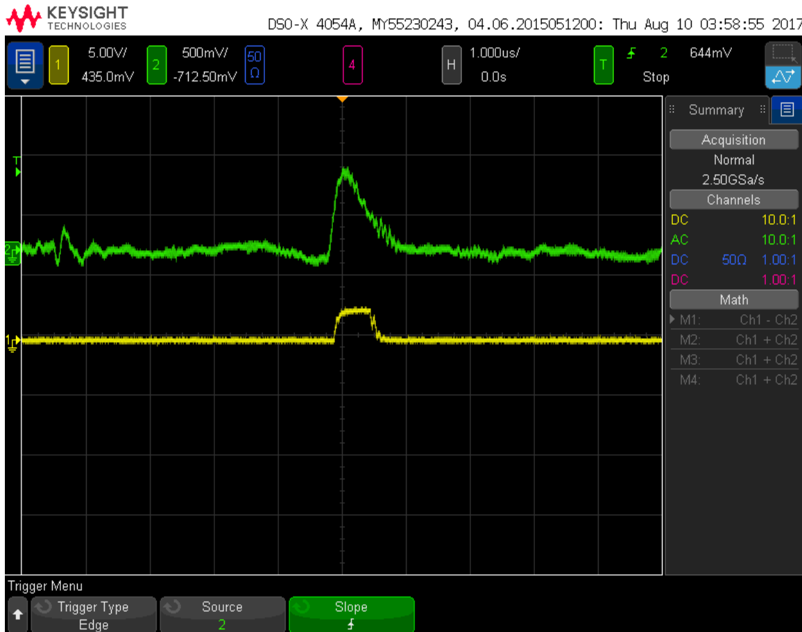
Figure A.3: The response to a beta particle causing an event in the silicon strip detector. Channel 2 is the analog response and channel 1 is half of the LVDS signal.
