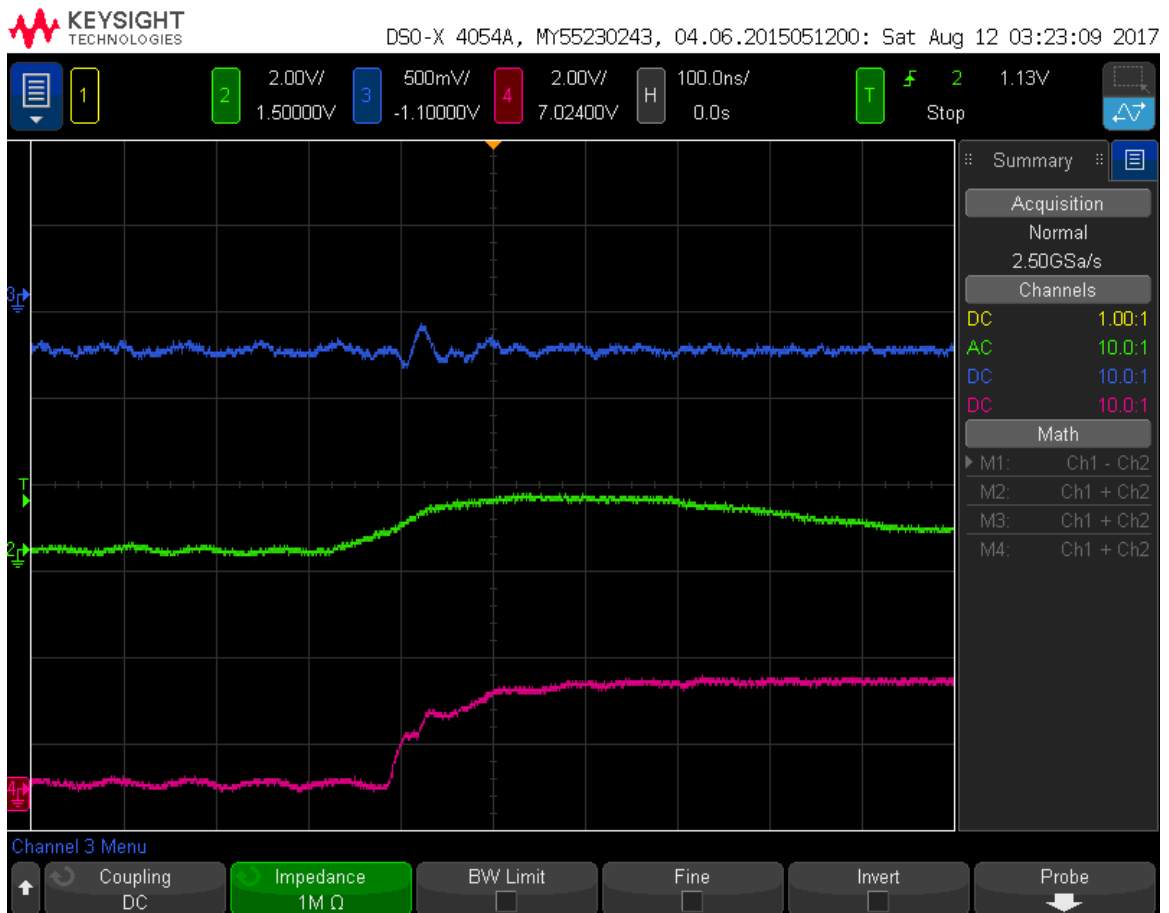
Figure 3.7: The QWAD response to a beta particle event from a silicon strip detector. Channel 3 is the silicon detector response measured at the point as it enters the QWAD, channel 2 is the analog response from the QWAD amplifiers, and channel 4 is half of the LVDS response.
