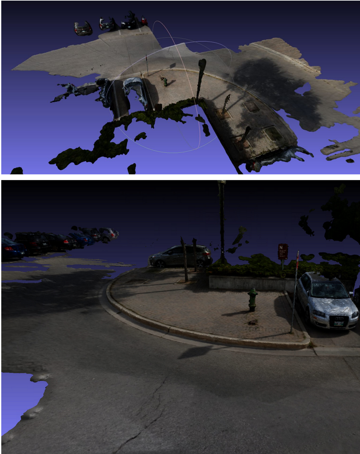
Figure 2.2: The final stage in photogrammetry converts a 3D mesh into a textured 3D representation of a scene.
