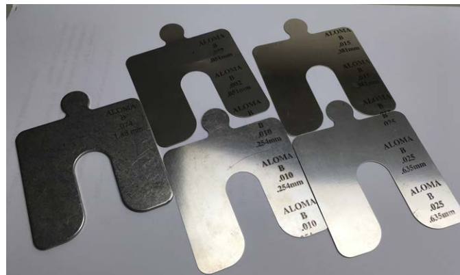
Figure 3.3. A set of the steel standard gauge blocks to determine the electrode separation of the CIGRÉ holder.
