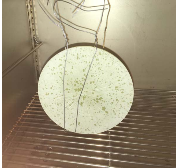
Figure 5.13. The FRP sample after 6 hours drying at 100 °C.
