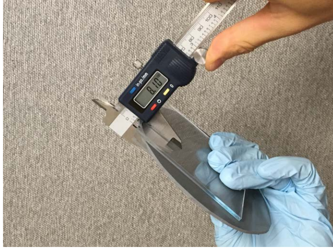
Figure 3.5. The method used to measure the sample thickness.
