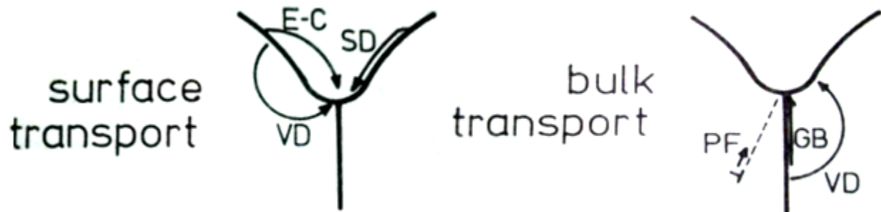
Figure 10: Diagram of surface and bulk transport mechanisms [2]
