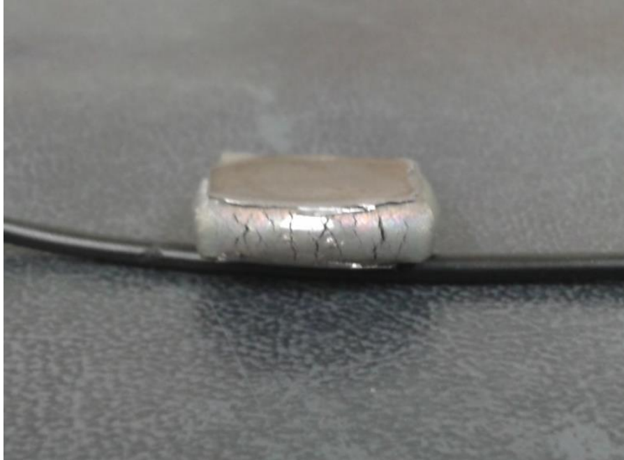
Figure 58: Representative Ruptured Sample Occurring at >30% Deformation at 1200°C
