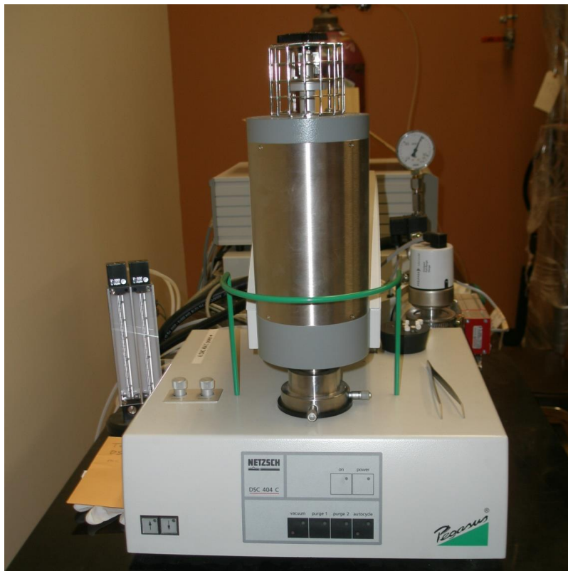
Figure 29: Netzsch DSC 404 C Differential Scanning Calorimeter used in this thesis
