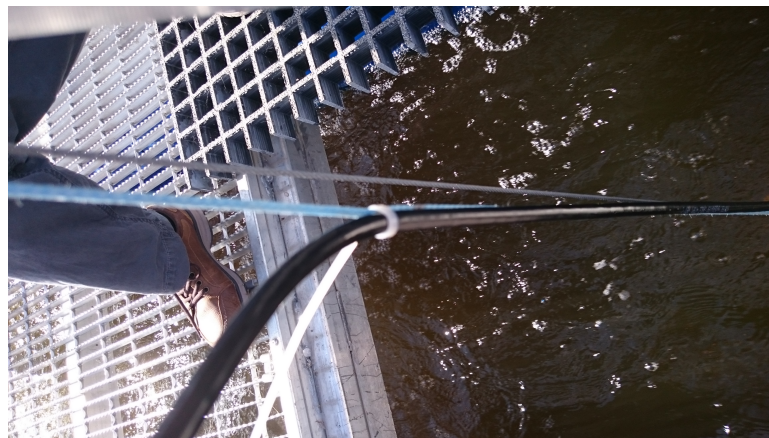
Figure 3.9: ADV data cable fastened to wire rope
