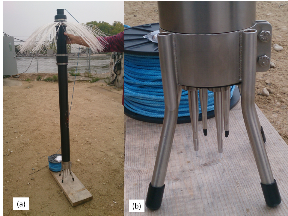
Figure 3.13: (a) Shear probe designed by RSI to be used in turbulence characterization (b) shear sensors which collect data as the instrument descends through the water column
