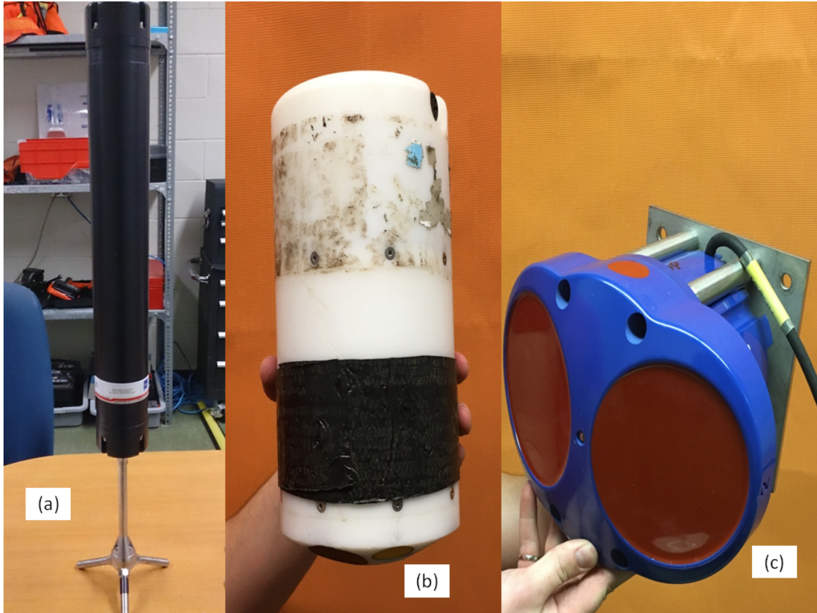
Figure 2.1: (a) ADV, (b) ADCP and (c) Horizontal ADCP instruments used in flow measurement. These acoustic devices are suitable for in-field river measurements.
