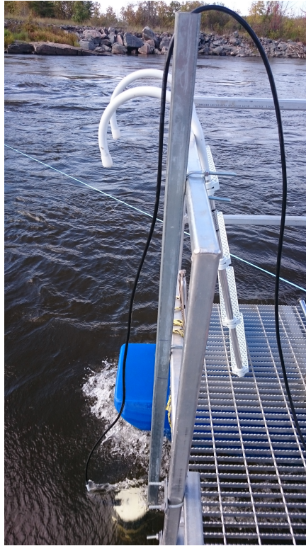
Figure 3.10: ADCP and channel fastened to the front of the measurement boat with U-bolts
