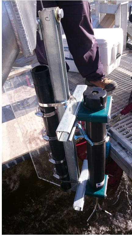
Figure 3.6: New ADV deployment unit fabricated from steel channel and clamps. To reduce operator requirements, a winch is installed to lower anchors (not shown). A rope is connected to the unit for operator-controlled placement of the unit in the water column.
