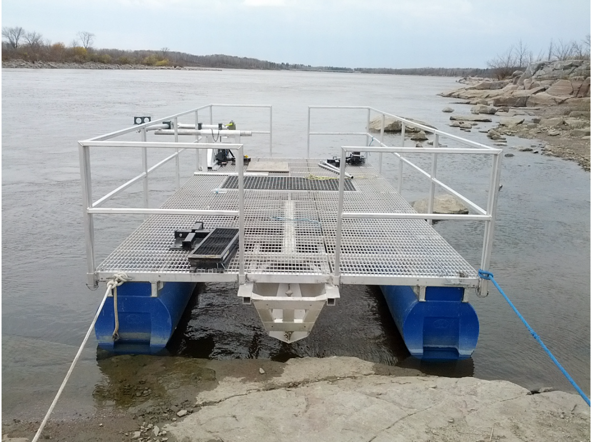
Figure 3.1: Fixed measurement platform used at the CHTTC without measurement instruments on the mounts.
