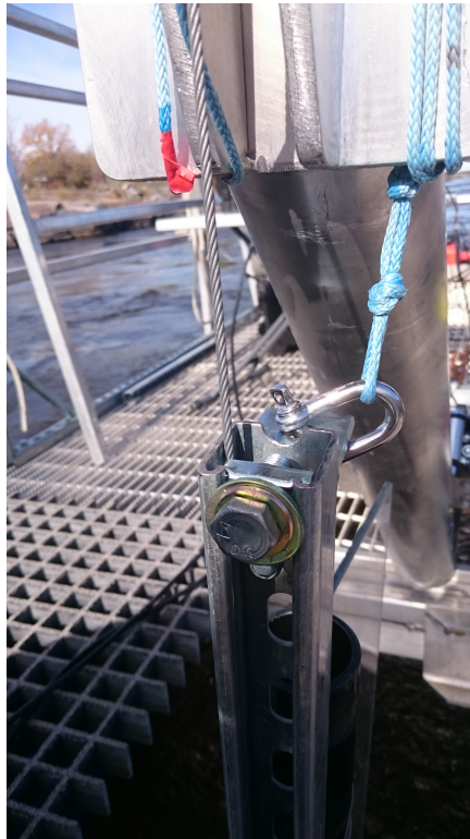
Figure 3.7: Amsteel blue rope fastened to ADV unit so as to allow the user to control the depth of the unit
