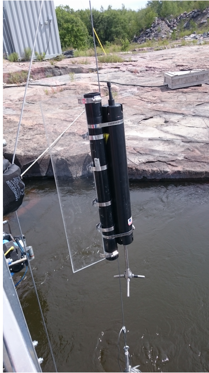
Figure 3.5: ADV first design using a cable pulley system about to be deployed in front of the fixed platform. Testing showed that instruments located in the front caused excess weight by operator and increased drag on the blue pontoon. A mid-section approach was then selected, along with a single guide wire to prevent cable entanglement.
