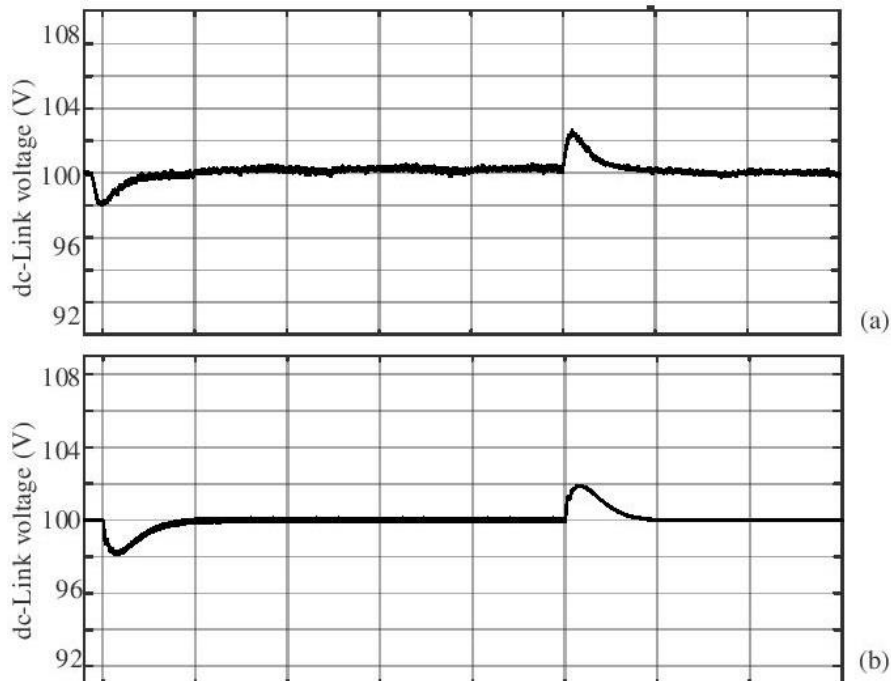
Figure 5.19: BESS dc-link voltage change upon a change in power set-point, (a) feed-back controller (experimental result, C_{dc-link} = 8800 \mu\text{F} ), (b) feed-back controller (EMTDC simulation, C_{dc-link} = 8800 \mu\text{F} ).
