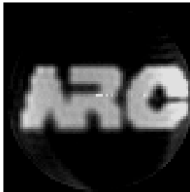
Figure 1.4 Demonstration of a small FOV excitation. Here the logo of the National Research Council of Canada (NRC) was generated in a water phantom using an eight-channel parallel transmit system.
