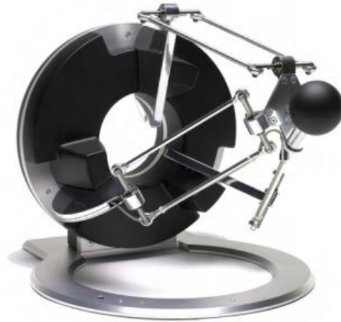
Fig. 3. Omega.3 haptic device (source: [24]).
