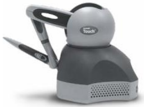
Fig. 2. Geomagic Touch, serial haptic device (source: [21]).
