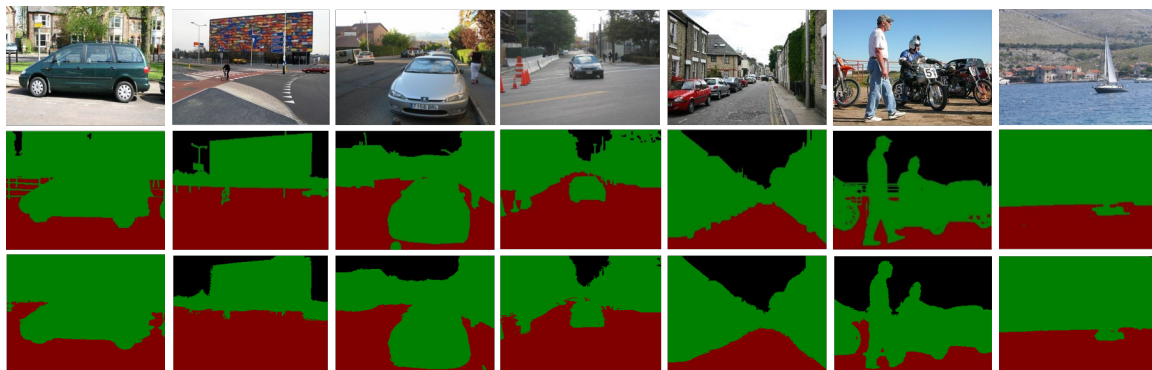
Figure 3.4: Sample results of geometric labeling on the Stanford background dataset [1]. 1st row: test images; 2nd row: ground-truth geometric labels; 3rd-row: geometric labeling results produced by ConvNet-CSVM2. Different geometric classes are represented by different colors.
