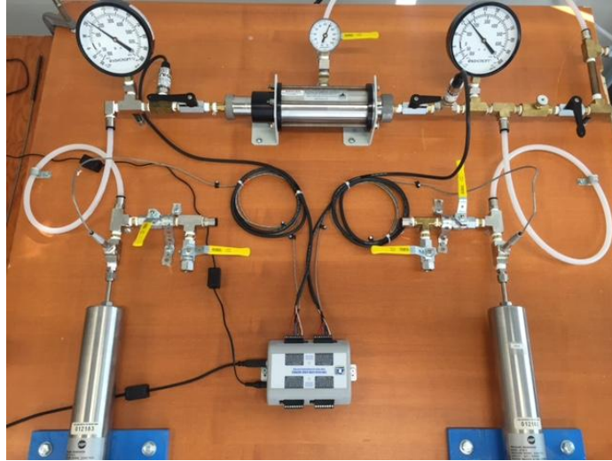
Figure 3-14: The modified pulse-decay experimentation apparatus.
