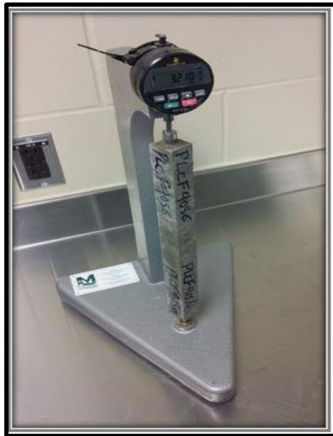
Figure 3.8: Length comparator utilized for determining the change in length of concrete prisms.
