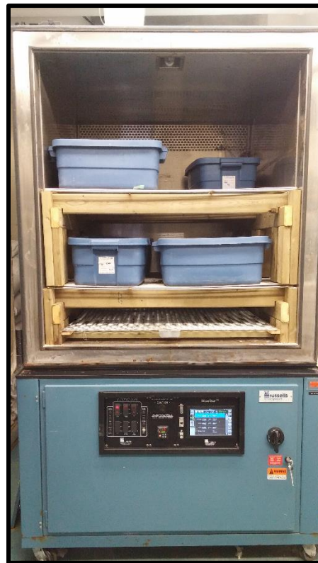
Figure 3.2: Environmental chamber used for F/T exposure.
