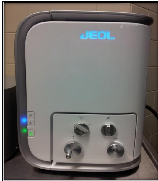
Figure 3.5: SEM sample chamber where the fracture pieces were mounted
