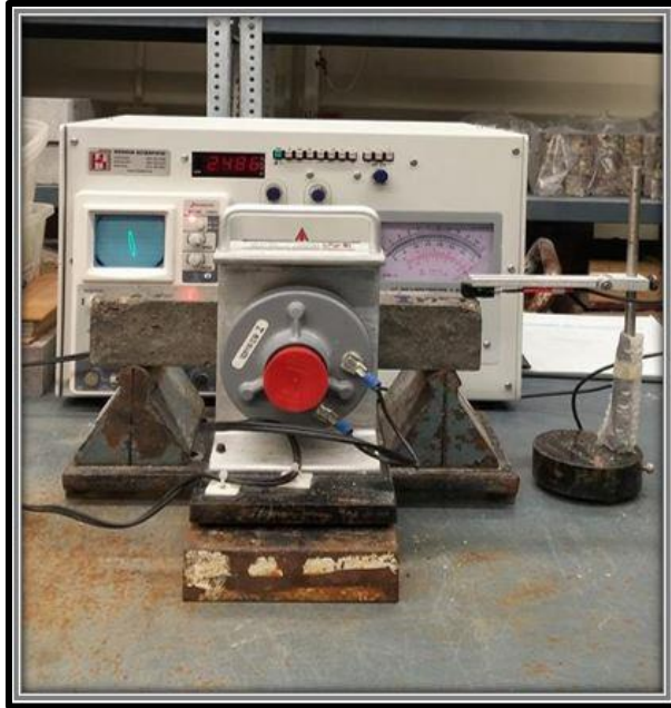
Figure 3.9: Sonometer apparatus used to determine the dynamic modulus of elasticity
