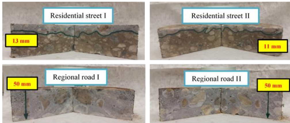
Figure 4.5: Whitish color showing the chloride penetration.
