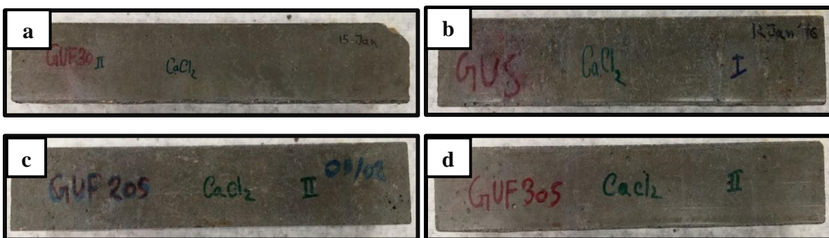
Figure 5.5: Intact specimens exposed to the CaCl_2 solution after 600 cycles: (a) GUF30, (b) GUS, (c) GUF20S and (d) GUF30S.
