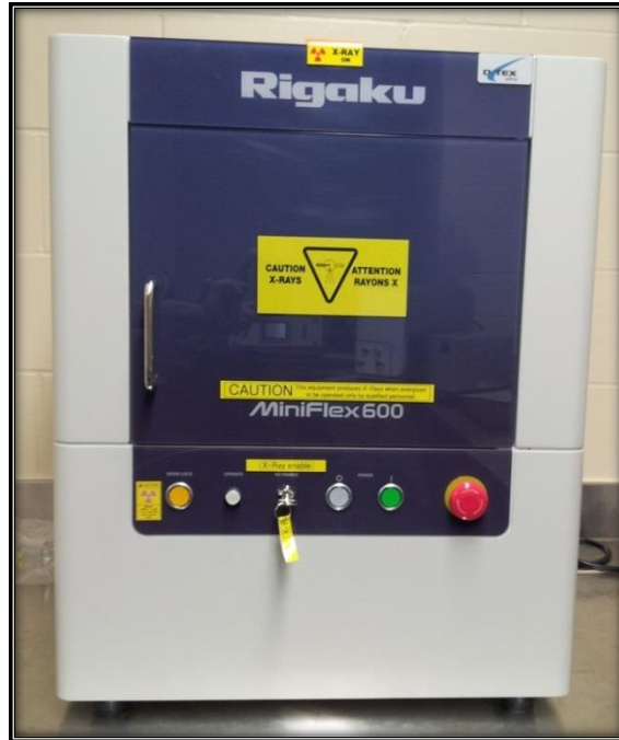
Figure 3.6: XRD instrument where the powder samples were mounted
