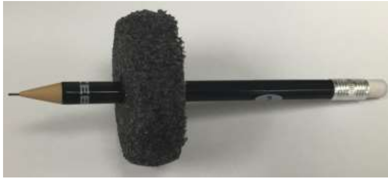
Figure 2. 4 Pencil-lead break test apparatus used in FRP test
