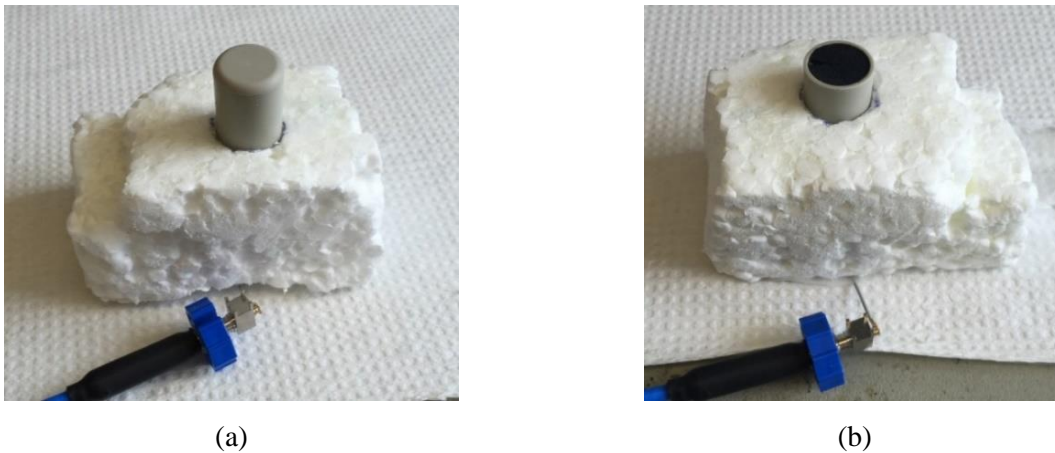
Figure A.1 (a) CSA Stubby mounted on styrofoam while under test. (b) Embedded CSA Stubby mounted on styrofoam under test.
