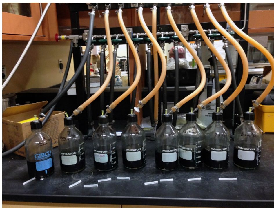
Fig. 2.4: Purging N2 gas to provide anaerobic condition
