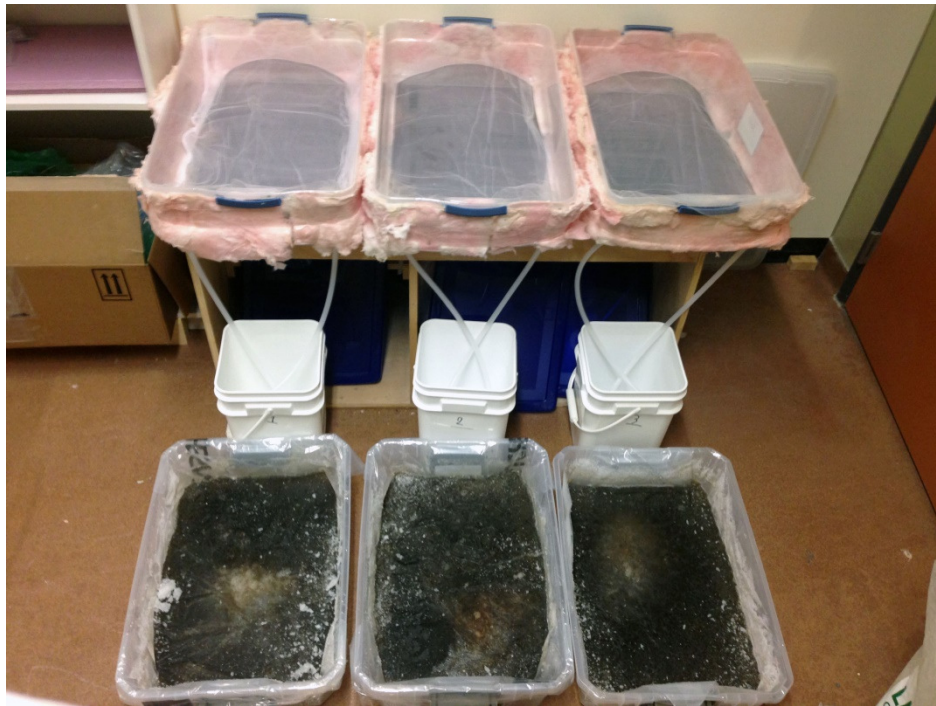
Fig. 2.3: Placing the frozen sludge for thawing
