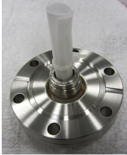
Figure 5.14: One of the HV feedthroughs being fit with the teflon shielding to block line of site between the pin and the grounded flange. The zip tie was used to help form the teflon and removed during installation.
