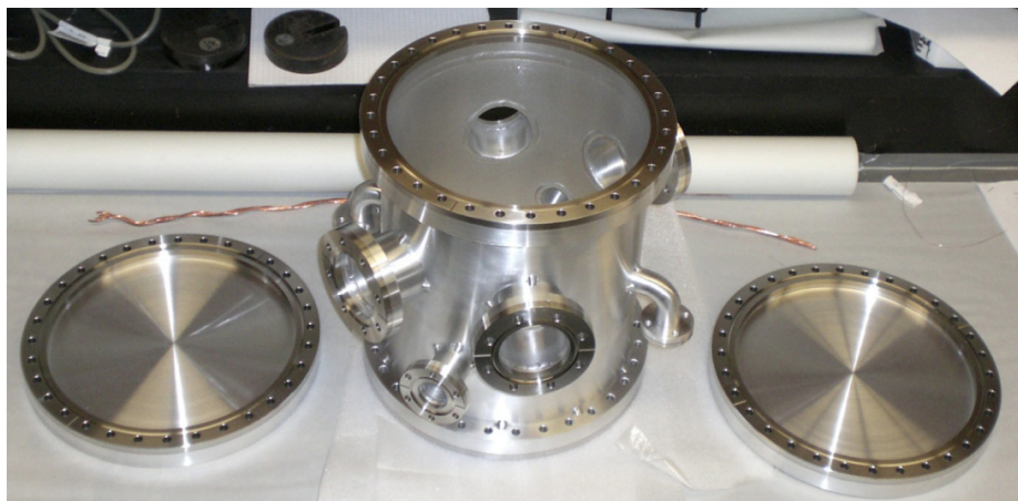
Figure 5.1: The aluminum target housing and end windows for the the n^3\text{He} target.
