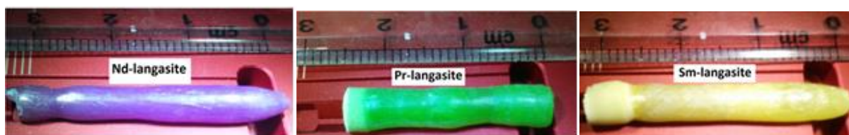
Figure 3.5 Single crystals of Be-langasites grown using floating zone image technique (left) \text{Nd}_3\text{Ga}_3\text{Ge}_2\text{BeO}_{14} , (middle) \text{Pr}_3\text{Ga}_3\text{Ge}_2\text{BeO}_{14} and (right) \text{Sm}_3\text{Ga}_3\text{Ge}_2\text{BeO}_{14} .
