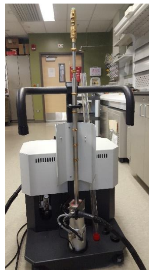
Figure 2. 8 Vibrating Sample Magnetometer by Quantum Design.
