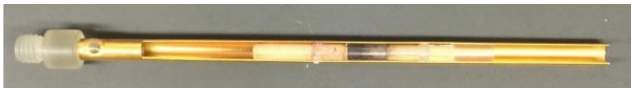
Figure 2.6 A non-magnetic brass trough with polypropylene sample holder. The magnetic response is generated only from the sample.
