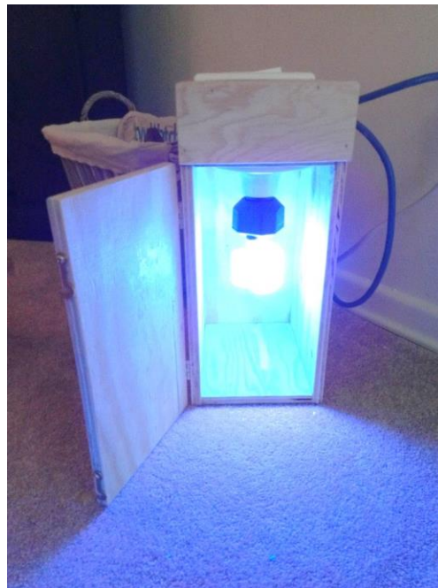
Figure 2: Ultraviolet light box used in this study
