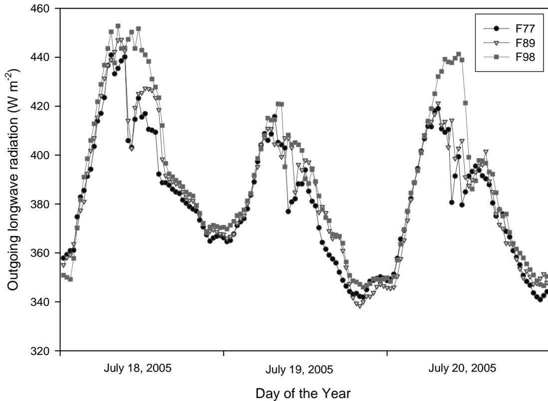
**Figure 2.2** Outgoing longwave radiation at three post-fire boreal forest sites burned in 1977(F77), 1989 (F89), and 1998 (F98) in central Saskatchewan. Points represent half-hourly values from July 18 - July 20, 2005.
