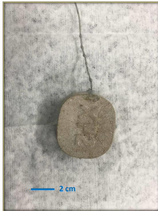
Figure 3.6: Zinc sacrificial anode used in this study.
