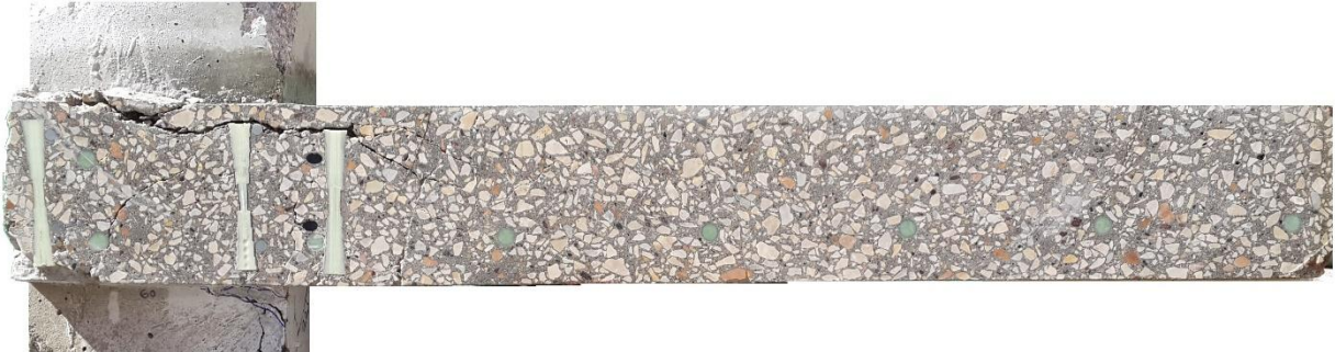
(a) Internal cracks for connection N-0.9-S8
