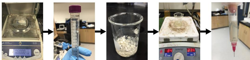
Figure 5-2 Alginate solution preparation process
