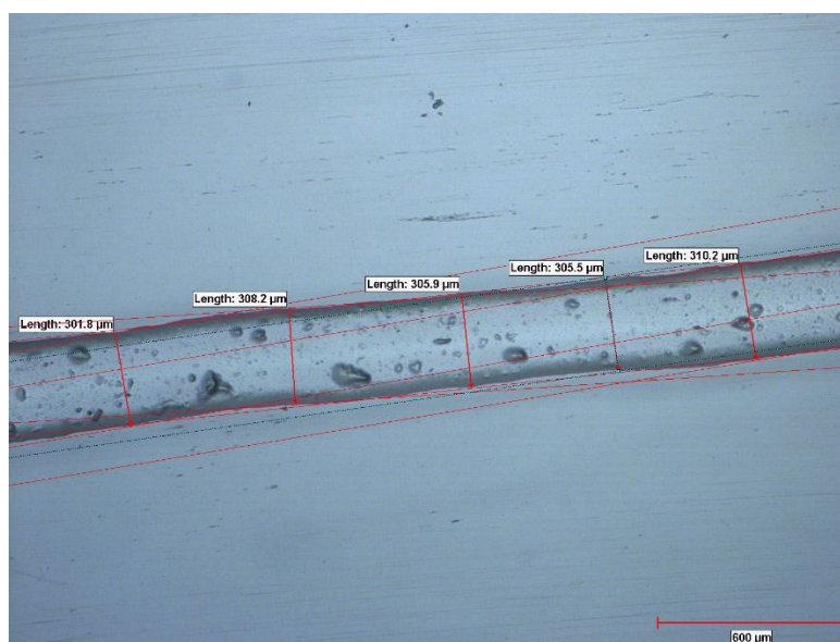
Figure 4-5. The measurement image of the strand using predicted parameter set
