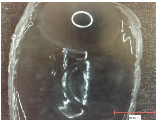
Nozzle 21g, pressure 20psi and speed 91mm/min
