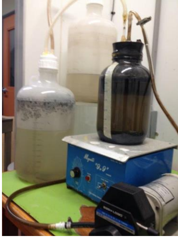
Figure 4- 4: Photograph of the semi-continuous anaerobic digester set-up.
