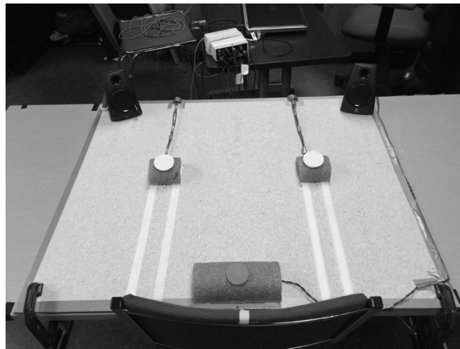
Figure 1. Superior view of the apparatus setup. The blue home switch is centred between the two yellow target switches (located 35.6cm from anterior edge of the surface). Two black Logitech speakers are placed behind the two target locations.
