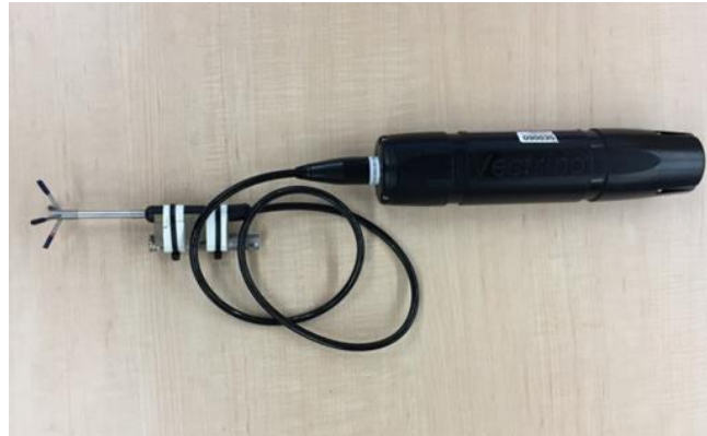
Figure 3-8: Down-looking ADV with cable probe.
