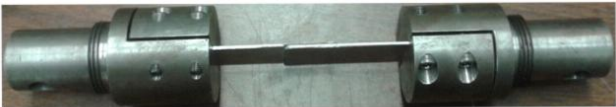
Figure 3.12: Test assembly of SLS test coupon
