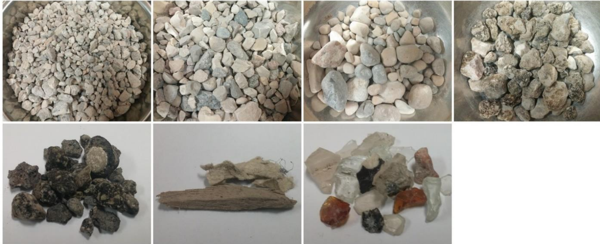
Figure 4-3 From left: First row- RCA material, Crushed Aggregates, Uncrushed Aggregates, Aggregate with other impurity; Second Row- Asphalt Coated Aggregate, Organic Impurity, Glass and Ceramic.
