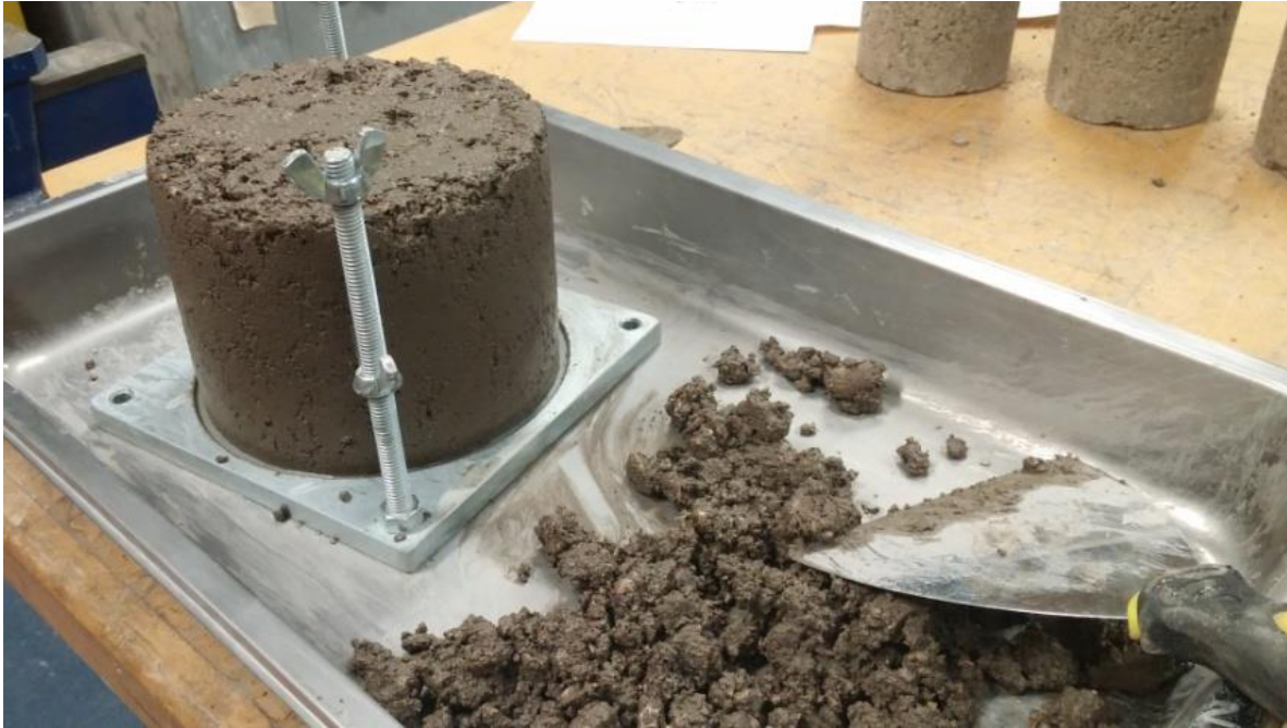
Figure 4-6 Extracted sample from the proctor mold after compaction.
