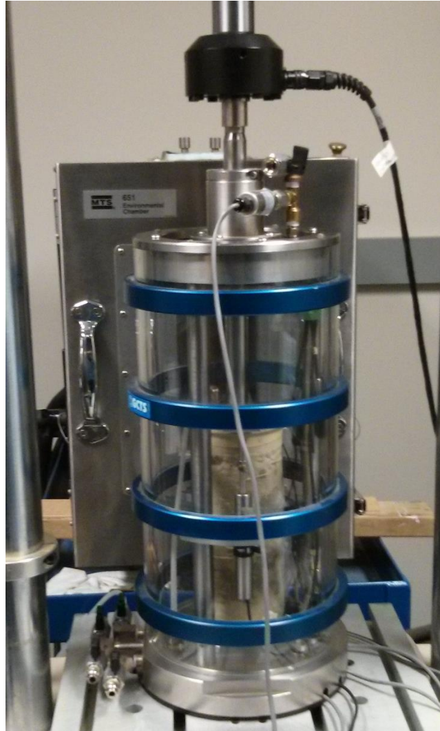
Figure 4-9 Resilient modulus test setup used for the research.
