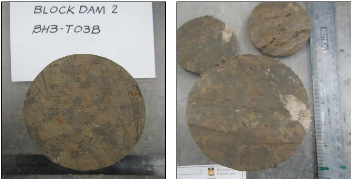
Figure 3-16. Clay core (left) and clay foundation (right) samples.
