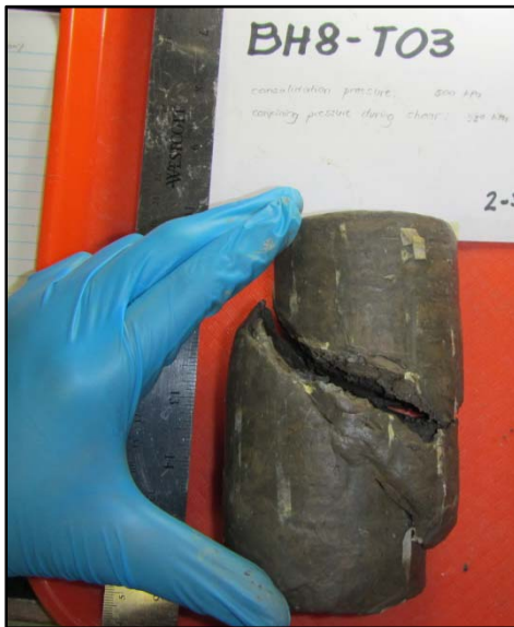
Figure 3-17. Clay core sample breaks easily along horizontal planes with silt lenses.
