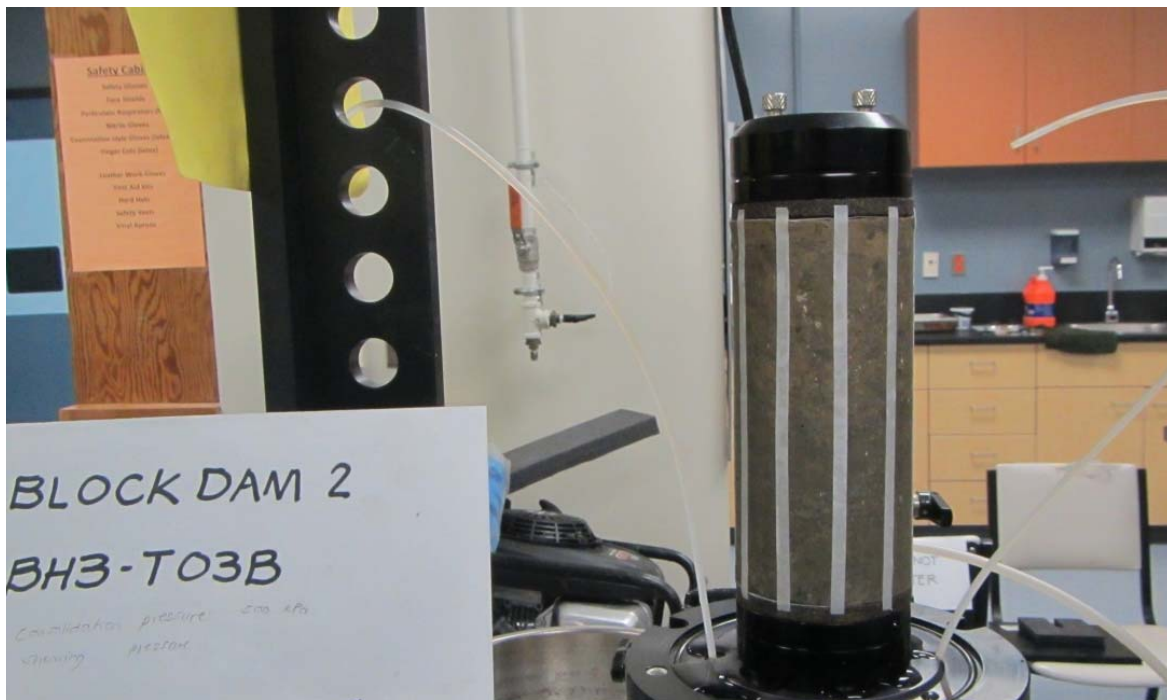
Figure 3-35. 71.12 mm diameter triaxial specimen from clay core.
