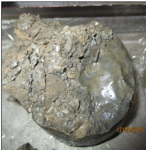
Figure 3-18. Polished fissures from clay core (left) and clay blanket (right) samples.
