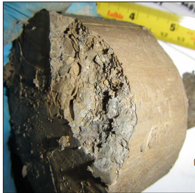
Figure 3-18. Polished fissures from clay core (left) and clay blanket (right) samples.
