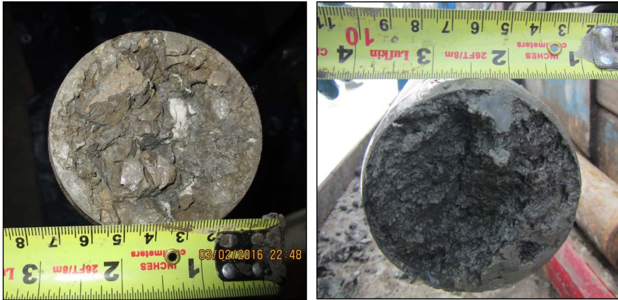
Figure 3-15. Off-shore samples. Fissured clay foundation at Section A-A (left), and soft clay blanket at Section B-B (right).
