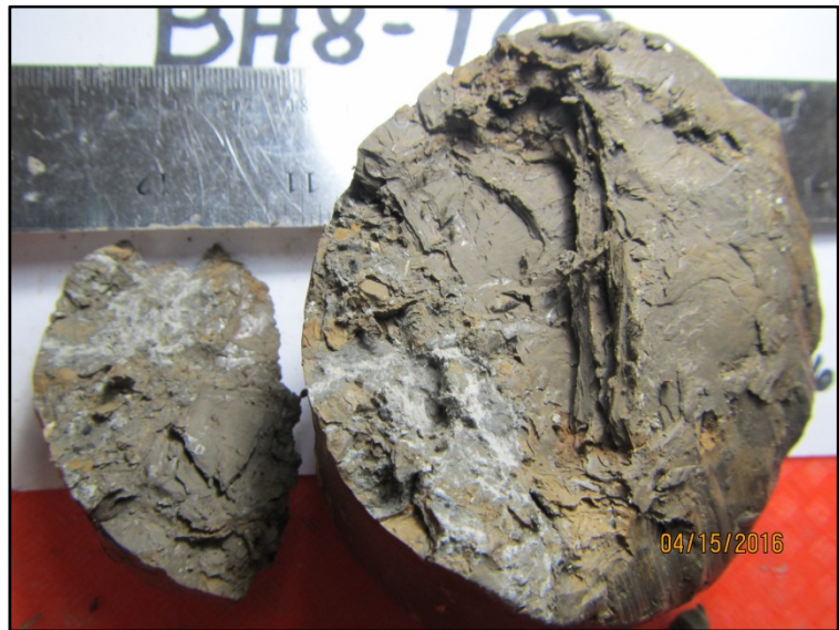
Figure 3-17. Clay core sample breaks easily along horizontal planes with silt lenses.
