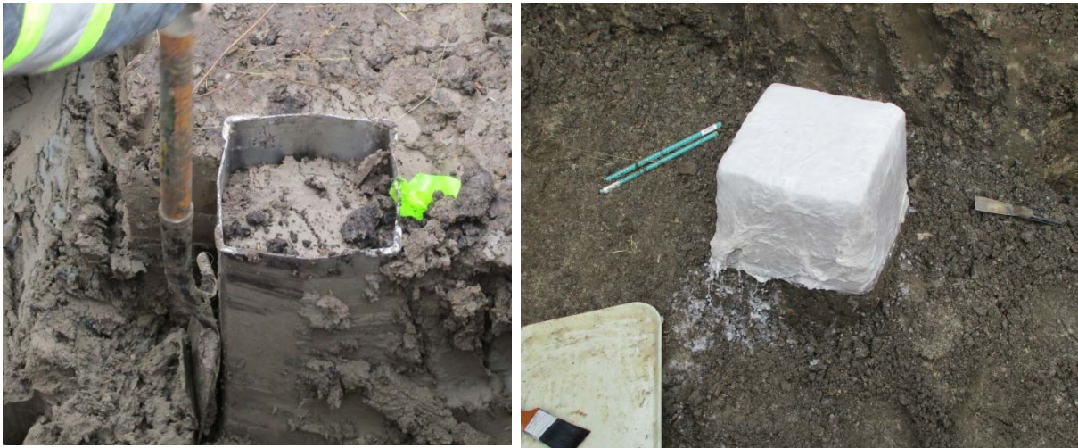
Figure 3-12. Block samples obtained using block sampler (left) and conventional method (right).
