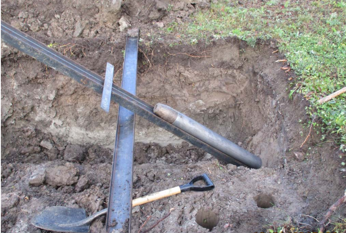
Figure 3-11. Inclined samples pushed into the test pit walls.
