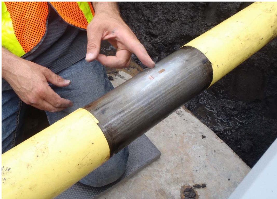
Figure 4-15 Epoxied Uniaxial Strain Gauge.
