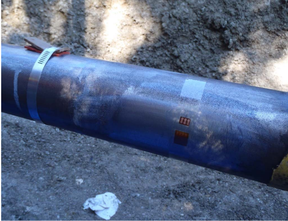
Figure 4-16 Epoxied Torsion Strain Gauge
