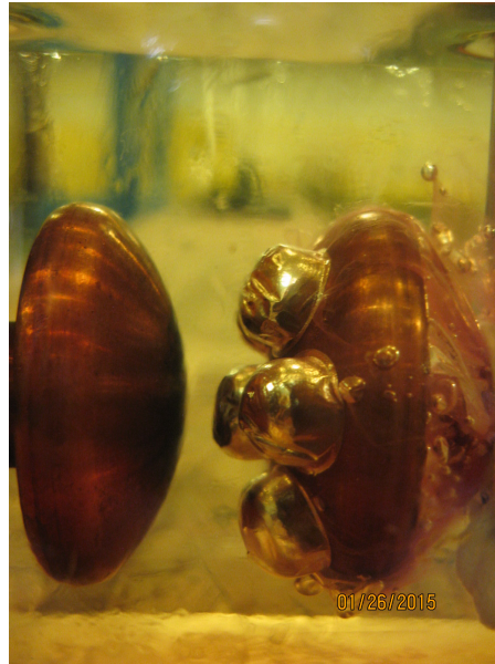
Fig. 4.11: The geometry of the test cell electrodes with bubble wrap (diameter of each bubble is 7 mm).
