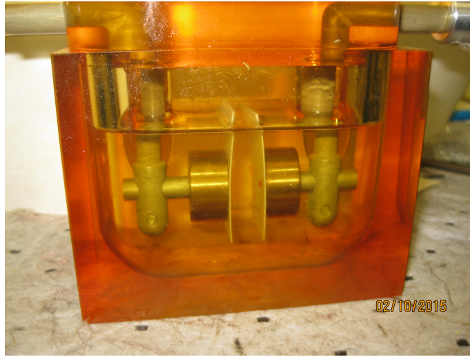
Fig. 4.12: The geometry of the test cell electrodes with floating metal particles (shavings).
