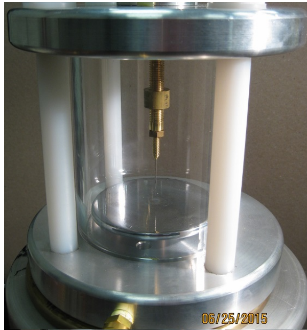
Fig. 4.5: Point-plane electrodes in air.
