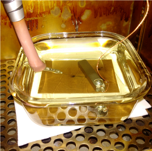
Fig. 4.22: Carbon tracks on the pressboard at 110°C after fault occurred.
