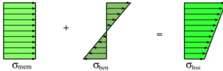
Figure 2- 1- 5 Stress distribution in front of weld toe according to the hot-spot stress [5].
