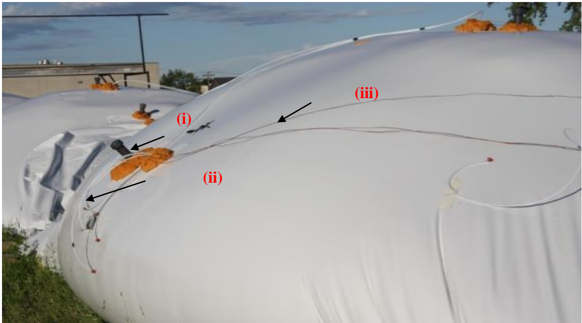
Figure 3.5 Silo bags with sampling arrangement (i) seed sampling ports, (ii) CO 2 sampling tubes, and (iii) thermocouples
