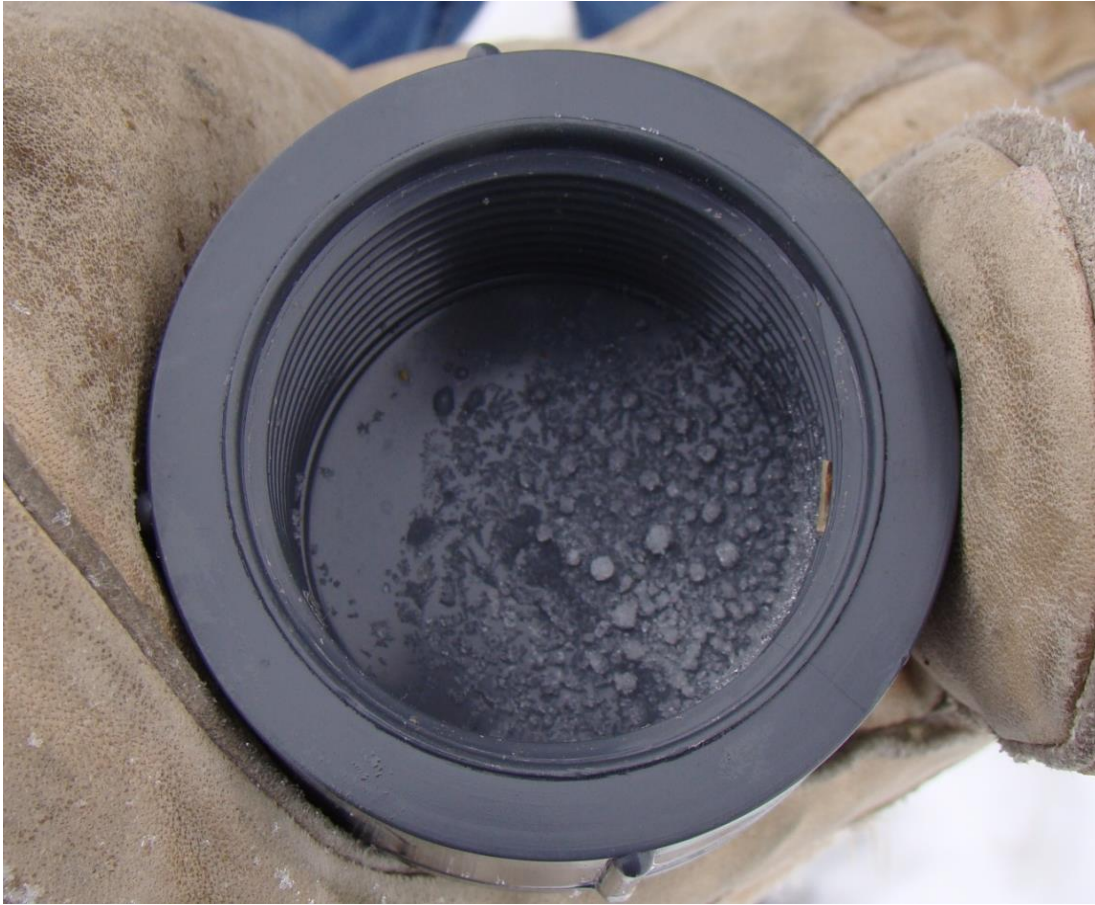
Figure 4.43 Condensation of water droplets at the sampling port cap during winter
