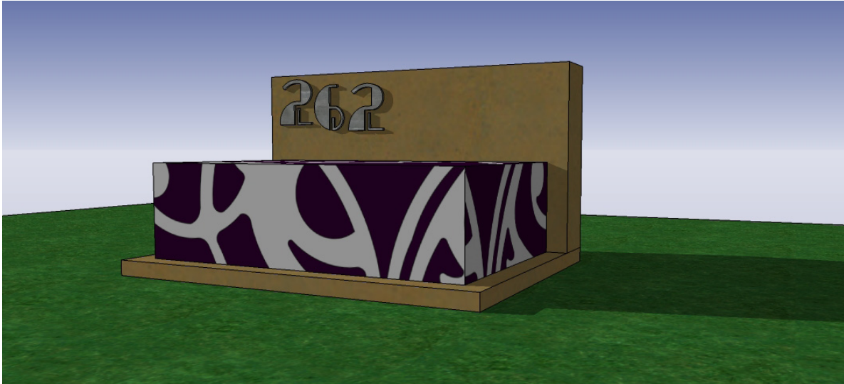
Figure 16.04 The legacy element. This component serves as a housing for utility lines after a demolition takes place. The cover can be painted in order to make it more appealing. An address set into the concrete denotes a sense of place and leaves a reminder of the past use of the lot and those who occupied it.
