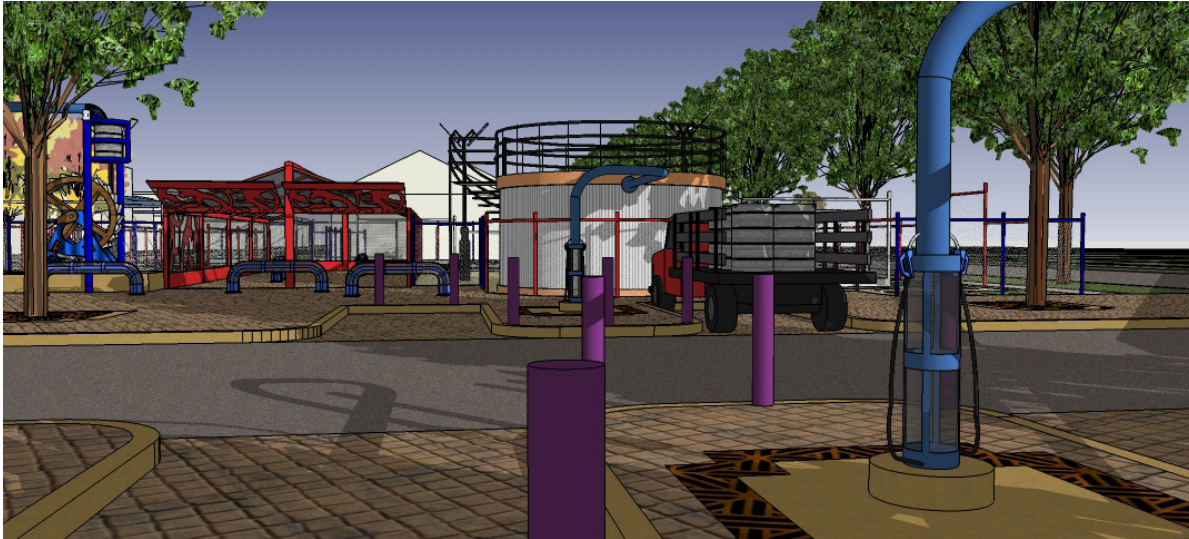
Figure 15.21 The connective pipe has an outlet where, similar to a vehicle service station, water can be pumped into barrels or a tank of the back of a truck. From here, water can be moved to and from garden sites when requested. Ideally this water could be accessed by anyone at any time, however in order to prevent tampering, the pumps would have to be shut off and secured until use.
