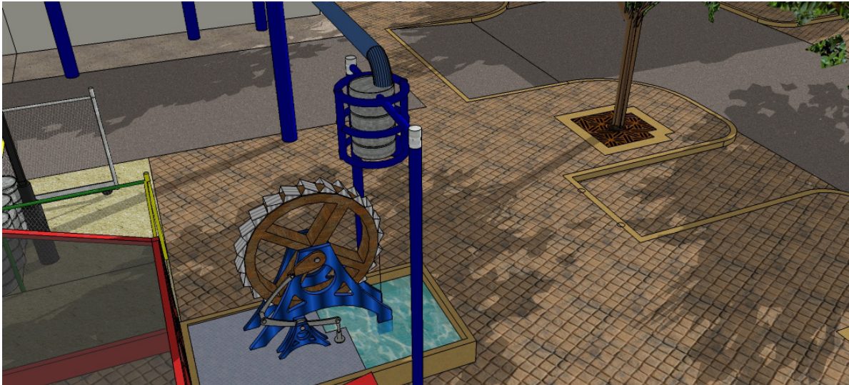
Figure 15.18 The water is channeled from the buildings to this point where it builds up in a barrel tank. This allows to water to fall with maximum pressure, over the waterwheel. The waterwheel is a simple and ancient mechanical device which can drive the pump in front. From here, the water is pumped from the basin below the wheel into a pipe filtration system.
