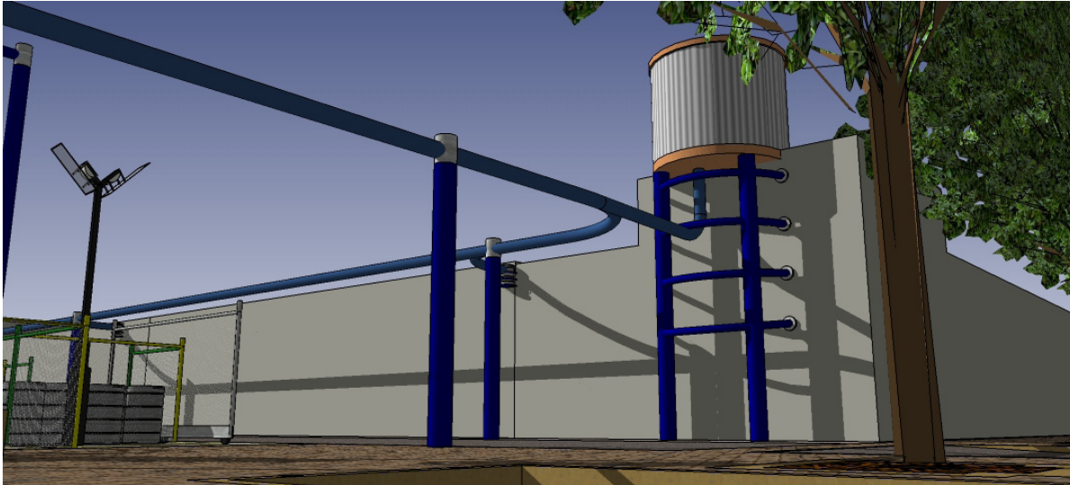
Figure 15.17 The building shown in this image is the back of a local laundromat. In an effort to link with existing context, a large reservoir is added here. Rainwater can be diverted to the laundromat's cistern if need be. Also, in some cases, grey water from the laundering process could supplement the gardens. This water would have to be drawn from machines that are regulated however and should be free of phosphates. Laundry water however, has been shown in many cases to be useable on crops, even those intended for consumption although in fairness, there are some limited risks involved.
