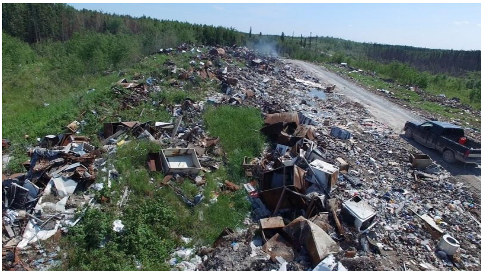
Figure 5.4: Road passes through the garbage dumpsite in Garden Hill. Waste materials are not compacted or covered and can be seen flying around the communities.
