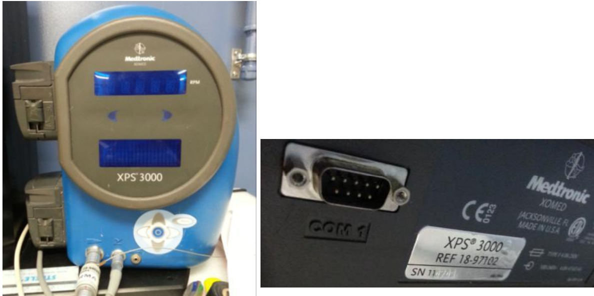
Figure 3-12: Medtronic XPS 3000 unit and its COM port on its back
