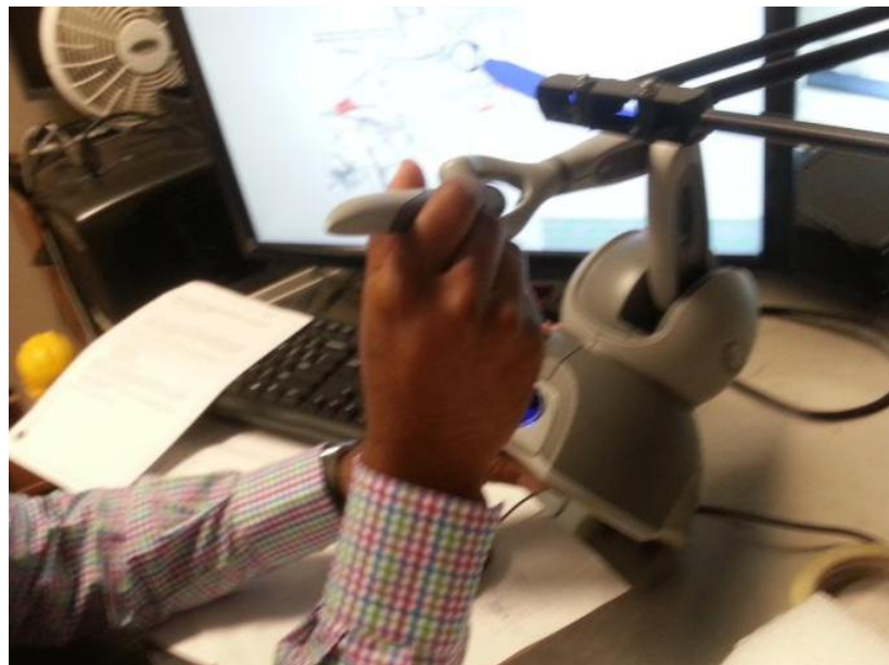
Figure 5-14: Participant forcing the Omni Phantom into a vertical orientation during evaluative testing
