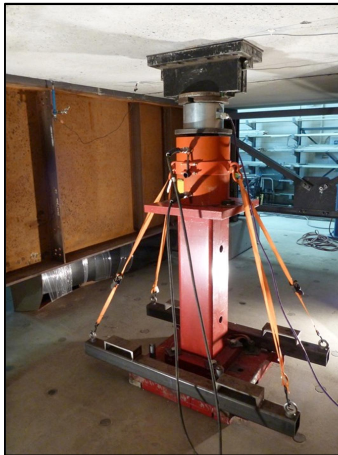
Figure 3-32 – Loading Apparatus for Static Tests (Tests #1 and #4)
