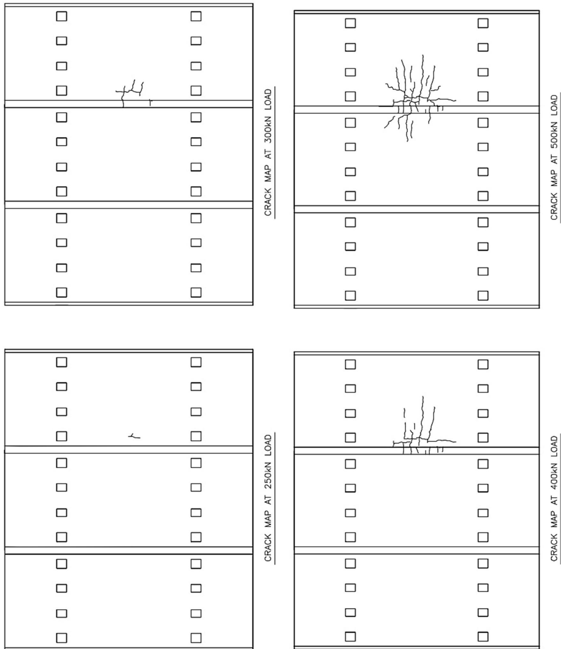
Figure 4-44 – Crack Progression from 250 kN to 500 kN (Test #4)
