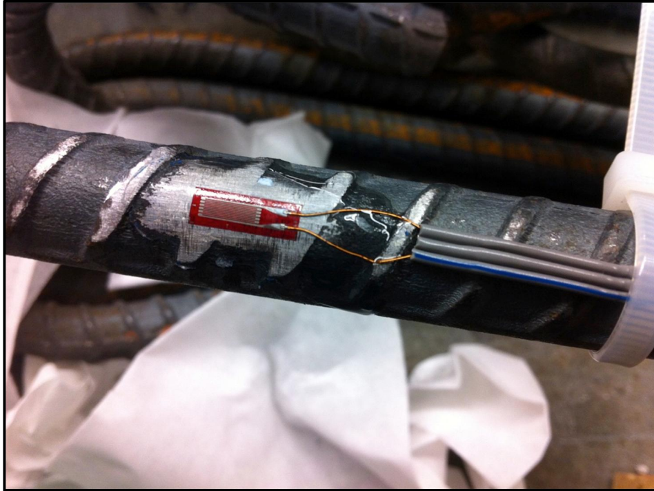
Figure 3-35 – ESG Adhered to Reinforcing Bar Prior to Coating (Typical)
