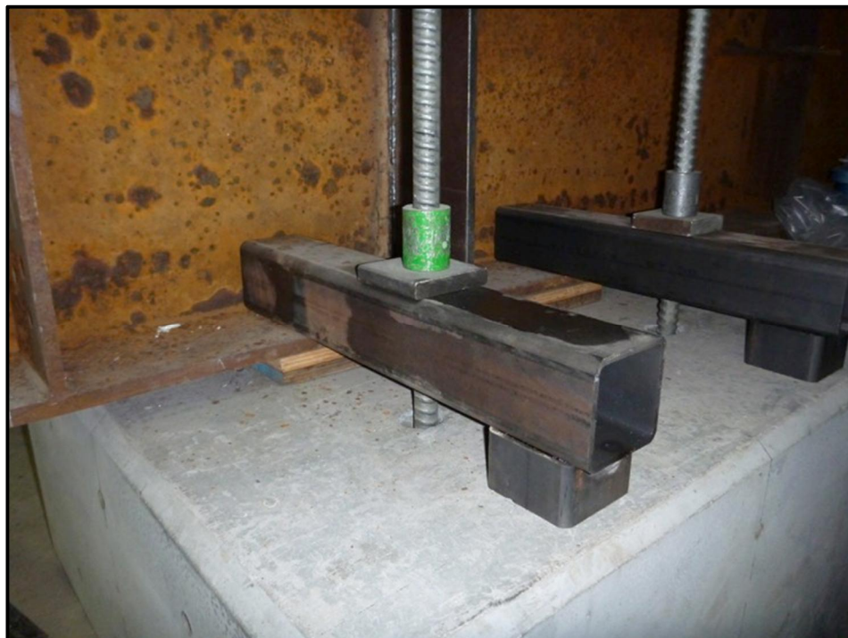
Figure 3-31 – Test Specimen Tie-downs on Interior of Girders
