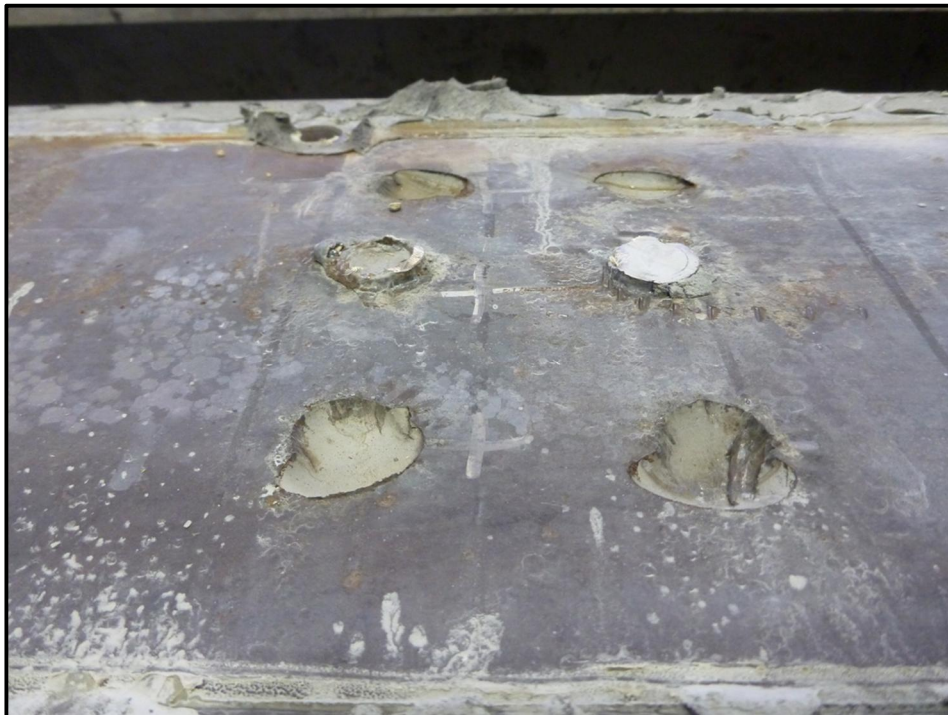
Figure 4-22 – Damaged Shear Studs In-Line with Loading Point (Test #2)
