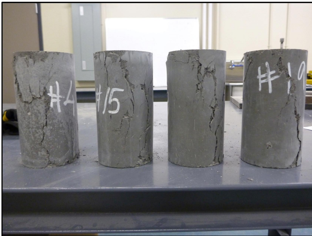
Figure 4-3 – Typical UHPC Failure Pattern
