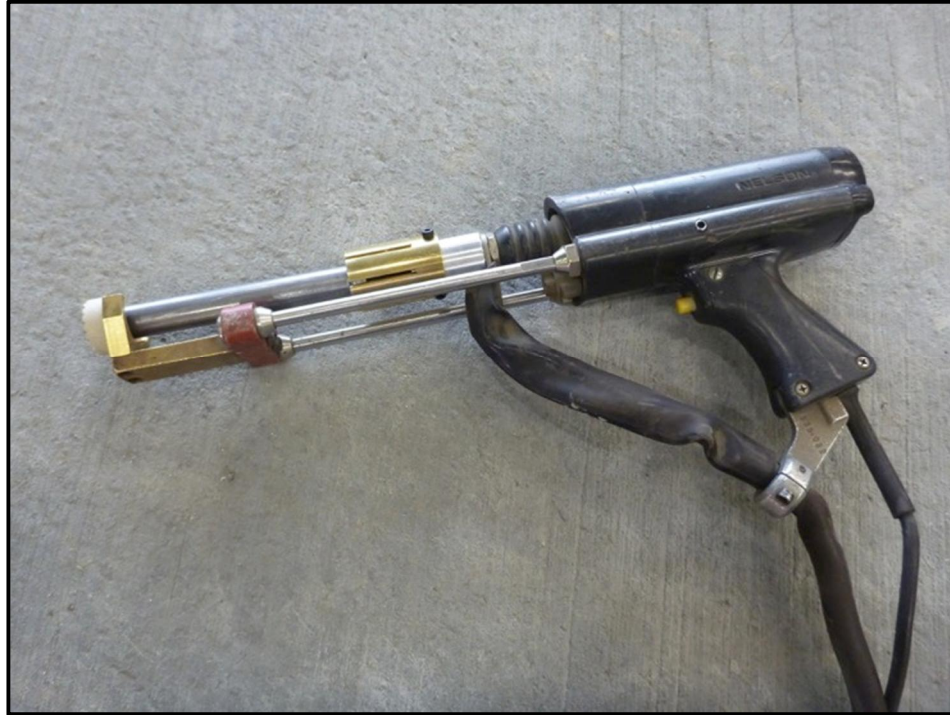
Figure 3-16 – Shear Stud Gun with Shear Stud and Ceramic Ferrule Loaded and Ready for Use
