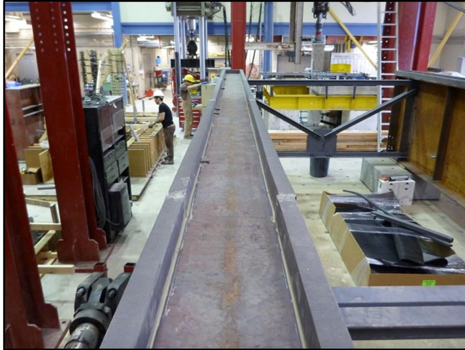
Figure 3-13 – EVA Foam Haunch Formwork (TS1) [Typical]
