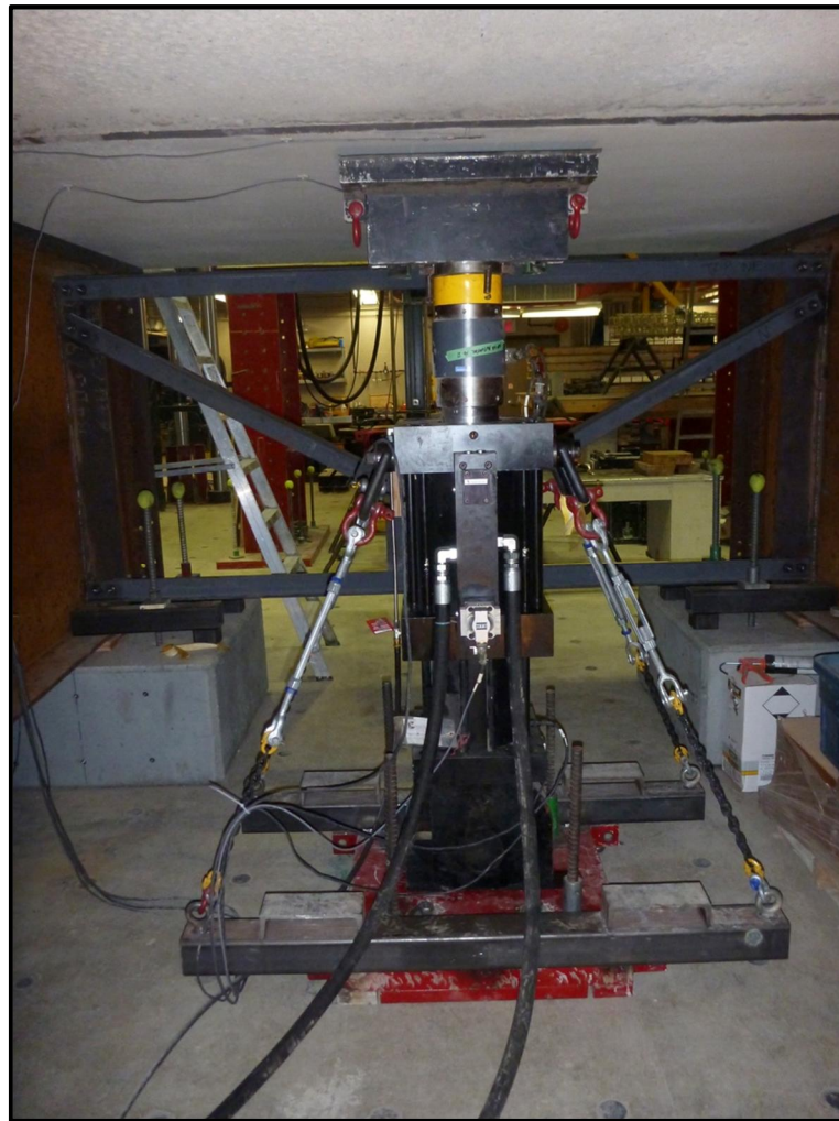
Figure 3-33 – Loading Apparatus for Fatigue Tests (Tests #2 and #3)
