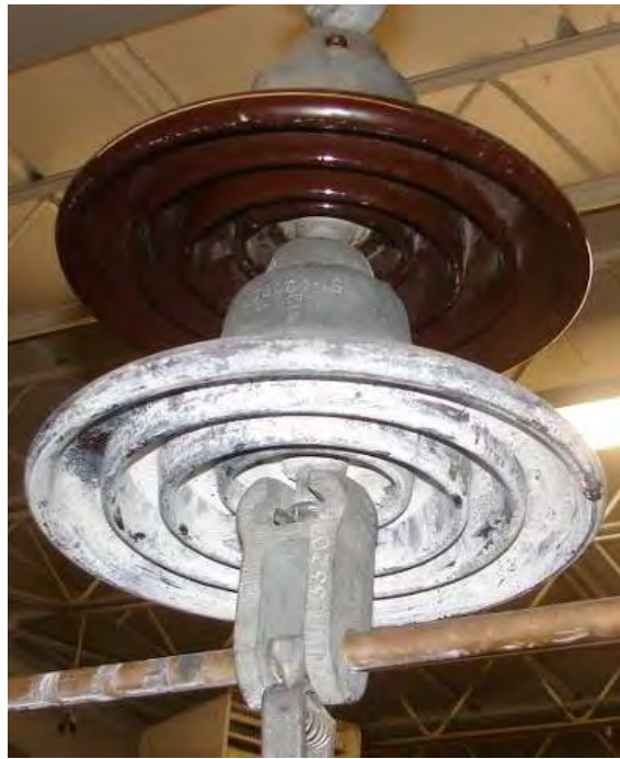
Figure 4.6: Contaminated insulator under the test; clean and healthy unit on top and contaminated unit at the bottom.
