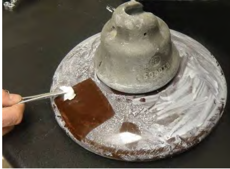
Figure 4.7: Measuring the ESDD level in the lab.
