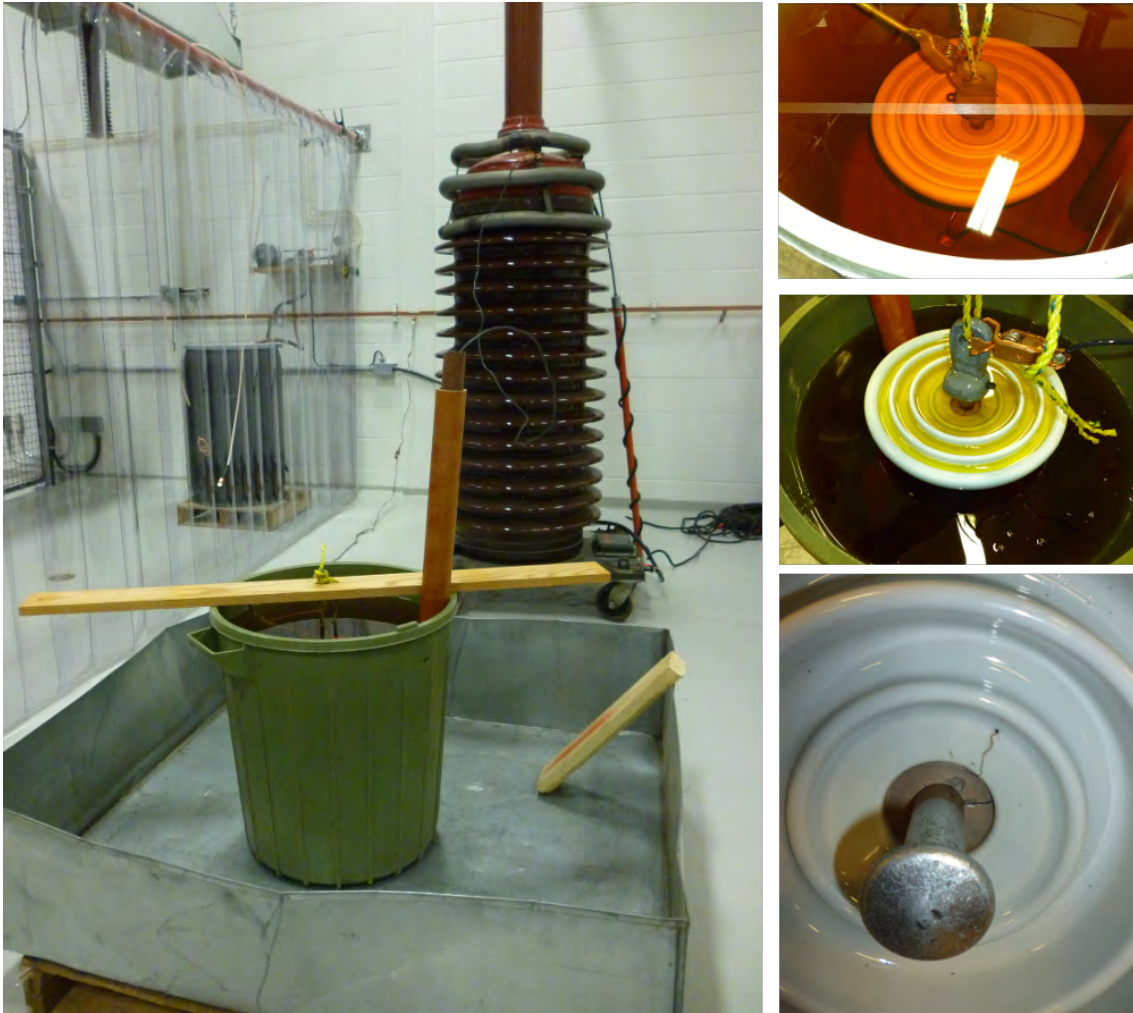
Figure 4.9: Puncture test arrangement using IEC 60383-1; test setup on left, insulator immersed in oil and under high voltage stress on top right, development of puncture on middle right, and punctured insulator ready to be tested for radiation signature on bottom right.
