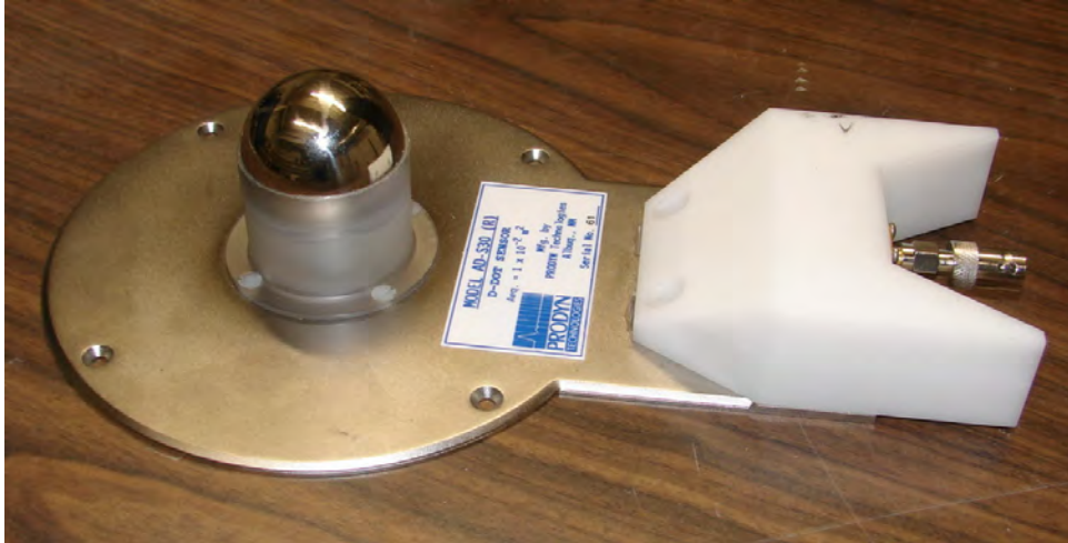
Figure 4.3: Prodyn's ACD-S30 Sensor.
