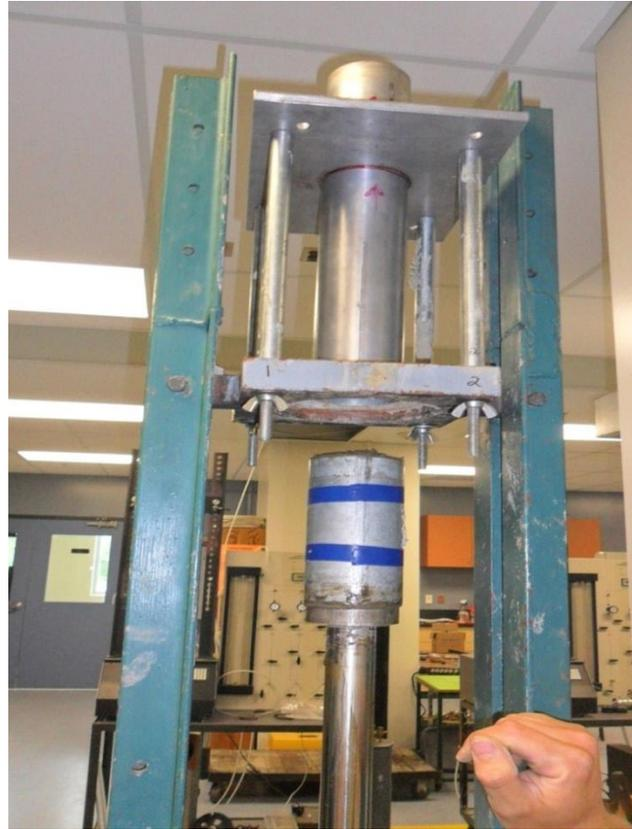
Figure 3.16: The electric jack device to put sample into the testing tube
