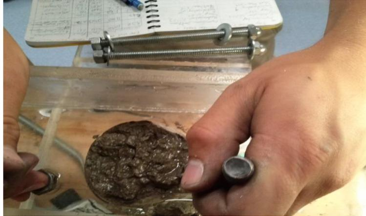
Figure 3.17: Soil sample preparation for EMD test
