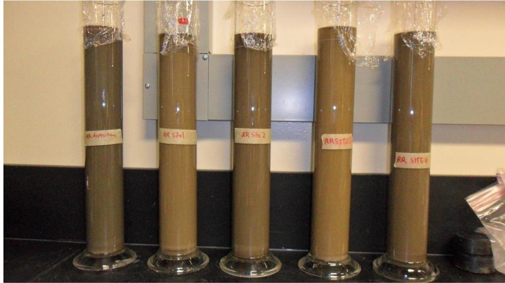
Figure 3.19: Hydrometry test to determine the fines particle size distribution
